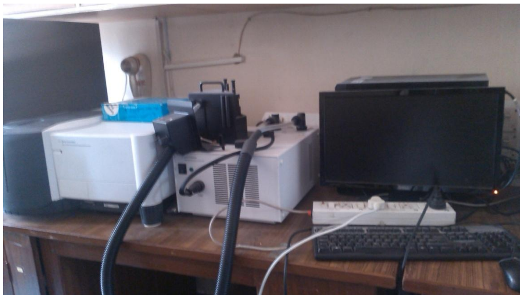
Fig 9: Photograph of experimental set up for PL spectrophotometer [model Cary Eclipse in material research lab]
