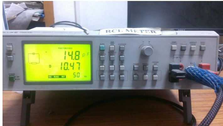
Fig 16: Programmable RCL meter [Model- FLUKE PM6306] for dielectric analysis
