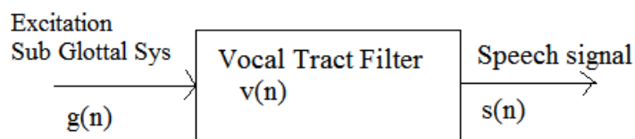
Fig. 1.6: Linear Acoustic model of Speech Production [11]
