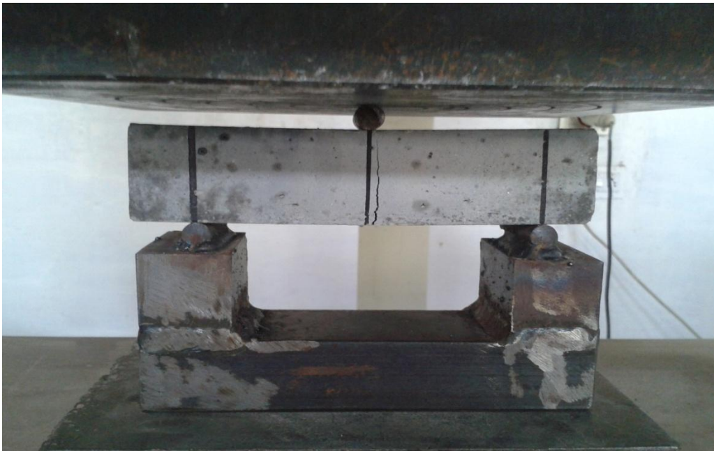
Fig : 3.4 flexure Strength test in progress.
