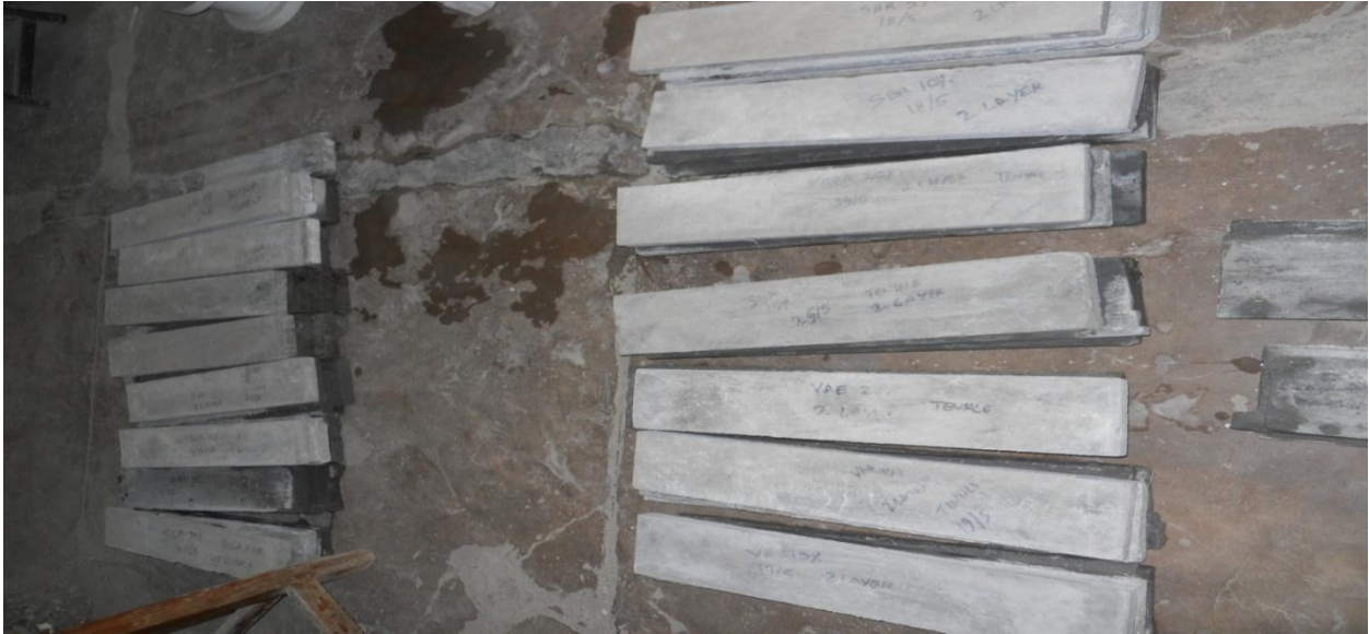
Figure : 3.9 Samples casted for tensile test.
