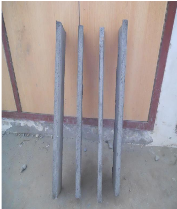
Figure : 3.6 a) Polymer modified ferrocement Beams after demoulding
