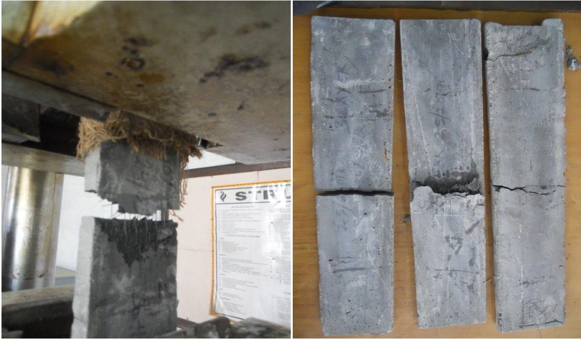
Figure : 3.10 Breaking and crack patterns during tensile test.
