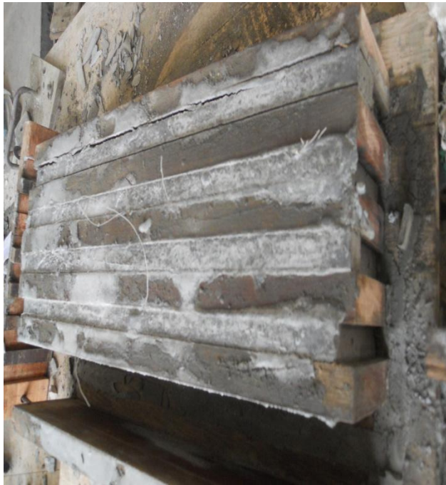
Figure : 3.6 b) Polymer modified ferrocement beams before demoulding.
