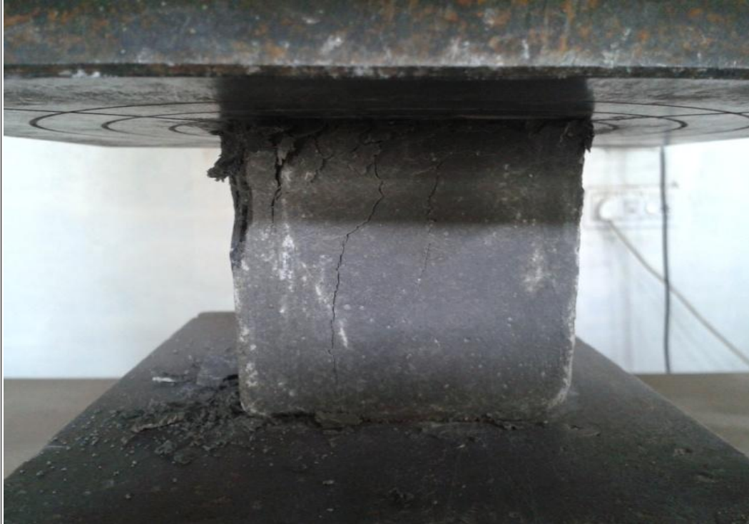
Figure : 3.3 Compressive Strength test in progress.
