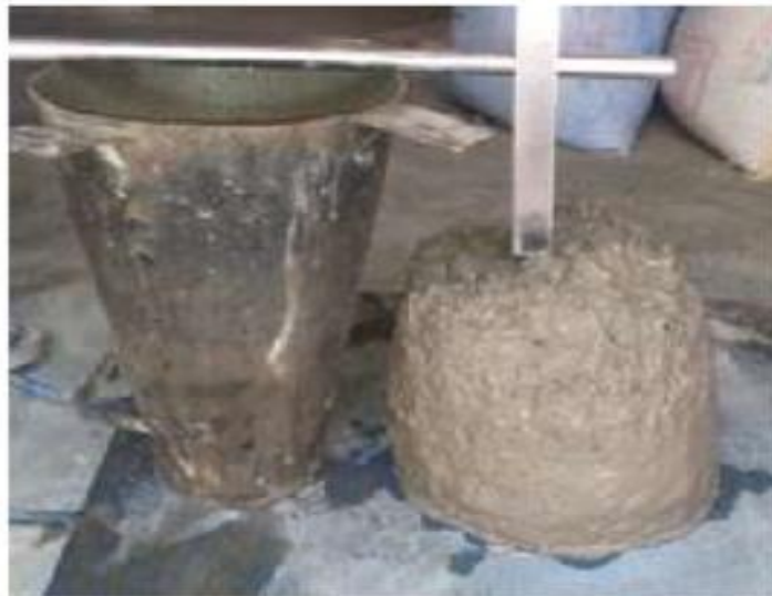
Figure 4.1: Showing the workability of concrete mix
