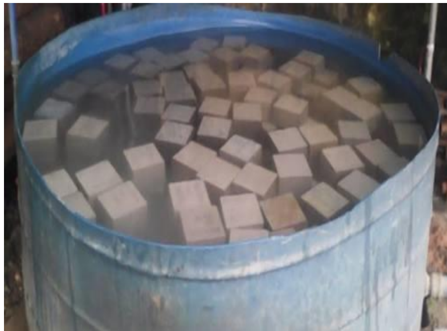
Figure 3.5: Cube specimens cured in water tank
