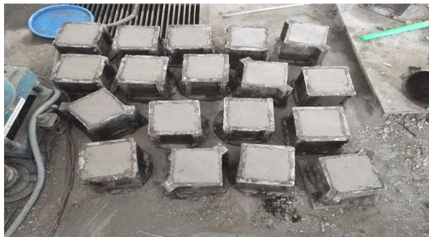
Figure 3.4: Finished mould containing GGBS concrete
