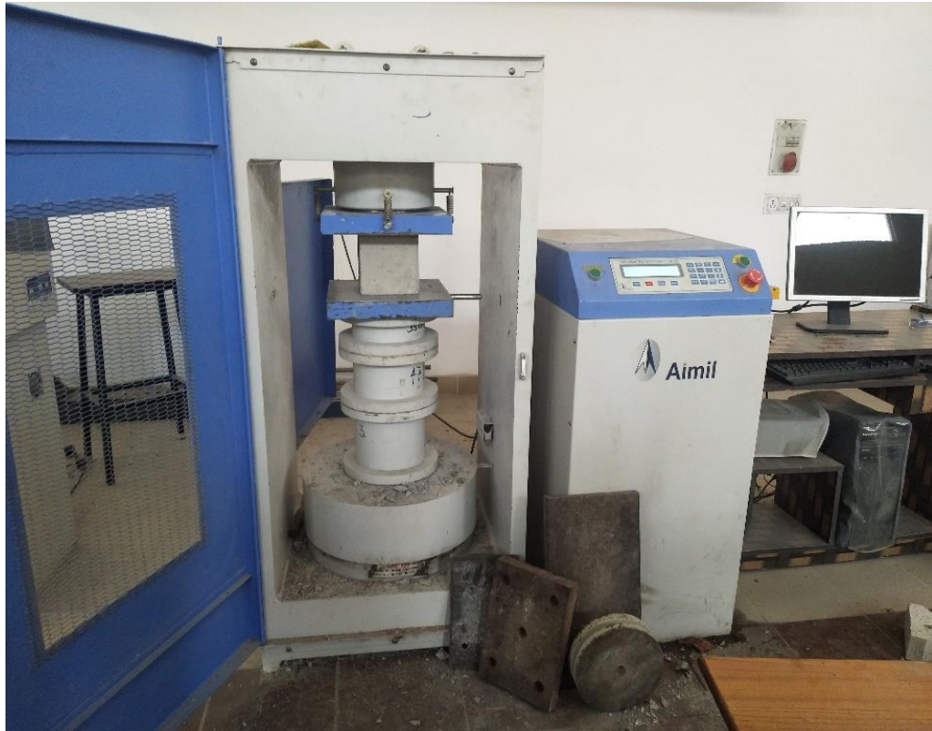
Figure 3.8: Cube under compression in Automatic Compression Testing Machine
