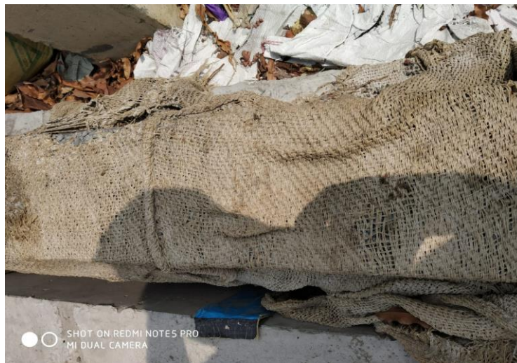
Figure 3.7: Cube specimens cured with wet burlap
