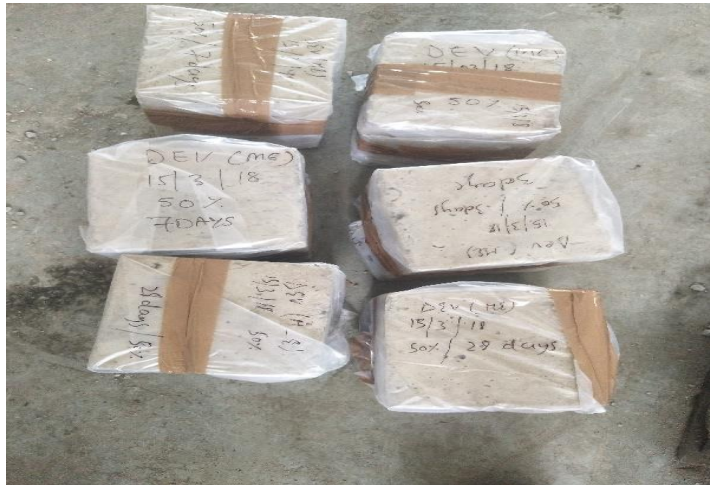
Figure 3.6: Cube specimens cured with fully sealed plastic sheet
