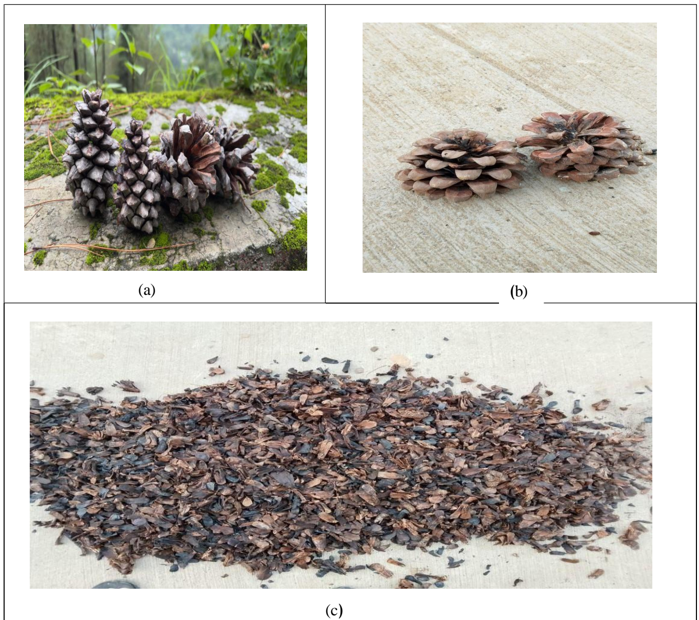
Fig.23 (a) Biomass(Conepine) Collected from forest. (b) Biomass after dried in Sun. (c) Biomass Chopped into small pieces.
