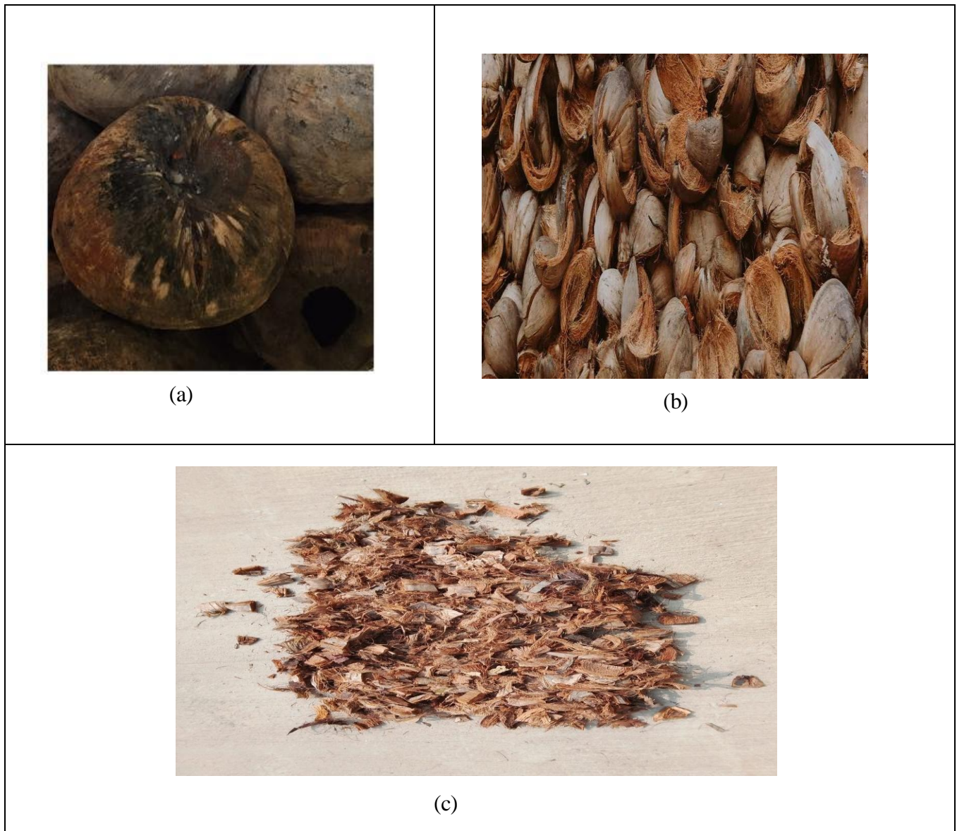
Fig.24 (a) Biomass(Coconutshell) Collected from Shop. (b) Biomass after dried in Sun. (c) Biomass Chopped into small pieces.
