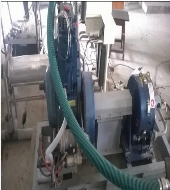
Fig.30 Dual fuel CI engine with variable CR
