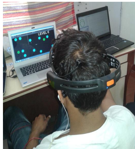
Figure 3.7 Experimental set up with subject while taking EEG signal
