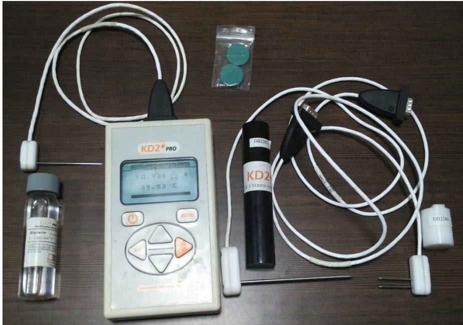
Fig. 3.9: Thermal Property Analyzer, KD2 Pro (Decagon Devices, Inc., USA)
