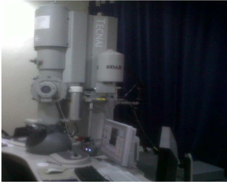
Fig. 3.8: High-Resolution Transmission Electron Microscope (HR-TEM)
