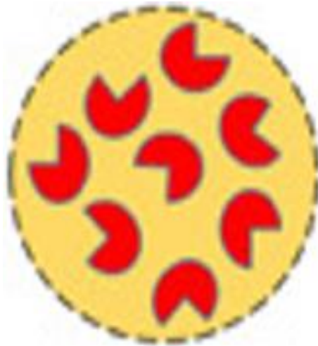
Figure 2.2 Entrapment of enzyme into the structure of MOF (Anboo et al., 2022)
