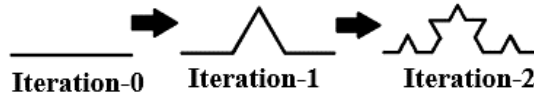
Figure 3.32 Design procedure for construction of the Koch curve fractal up to 2 nd iteration
