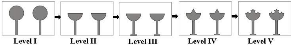
Figure 3.31 Intermediate design steps for the construction of final optimized fractal radiators
