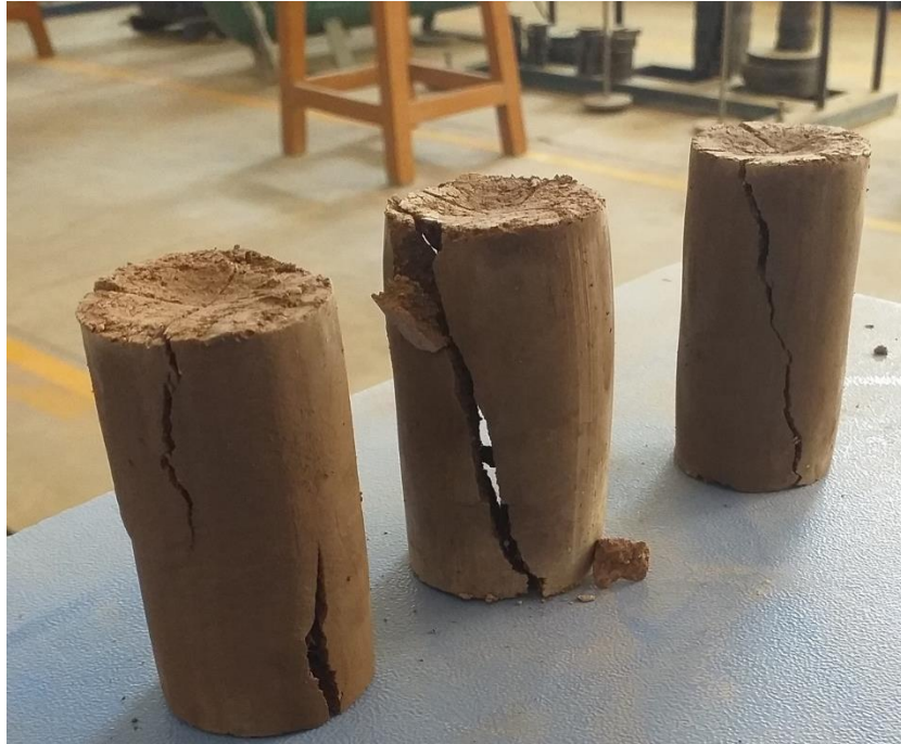
Figure 3.3 Failed sample of UCS
