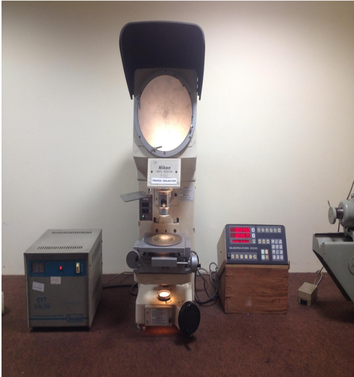
Figure 4.21: Nikon V10 profile projector
