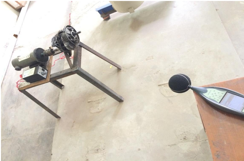
Figure 4.25: Measuring sound pressure level of gear box
