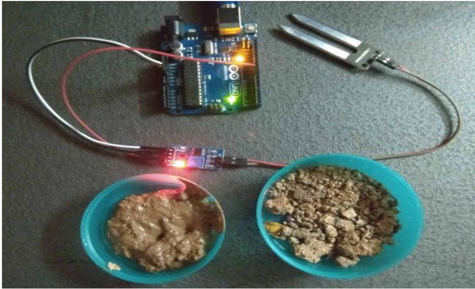
Figure 2.2: Fetching soil moisture information
