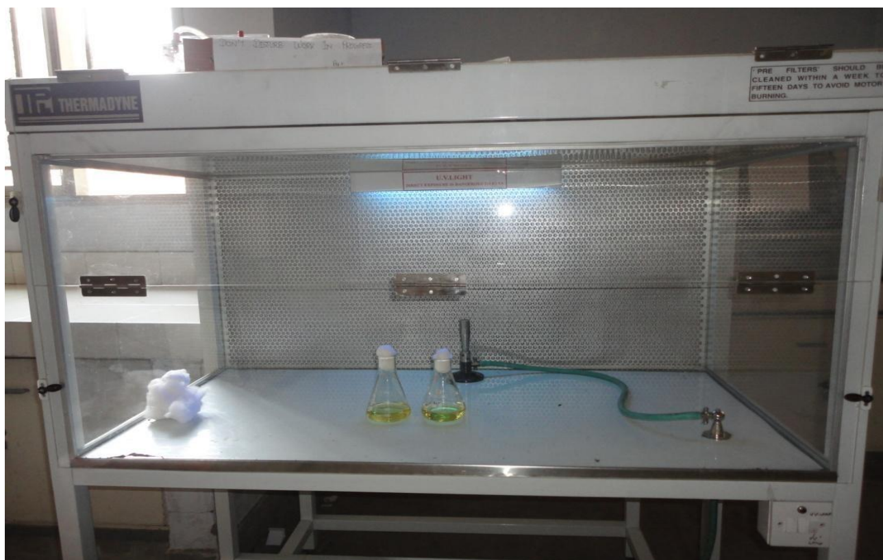
Figure 3.4 Laminar flow chamber
