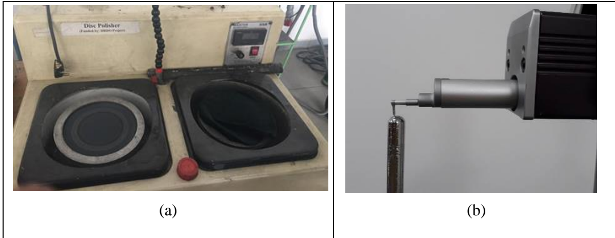
Figure 3.4: (a) Disc grinder & polisher (b) Surface roughness measured by stylus.
