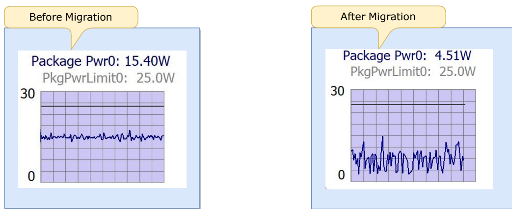
(a) Power Consumption Before Migration
