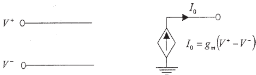
Fig 3.2 Ideal small signal equivalent of OTA[4]
