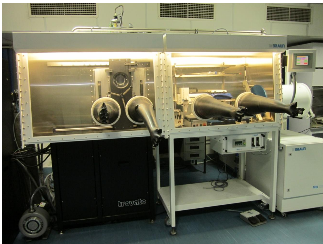
Figure 2.3: Glove box at NPL, New Delhi
