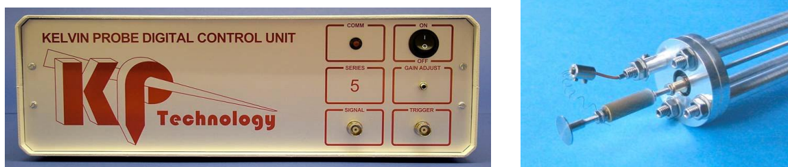
Fig. 2.8: UHV Kelvin probe head unit (right). The tip preamplifier is contained within the external and Digital Control Unit Front Panel (left).
