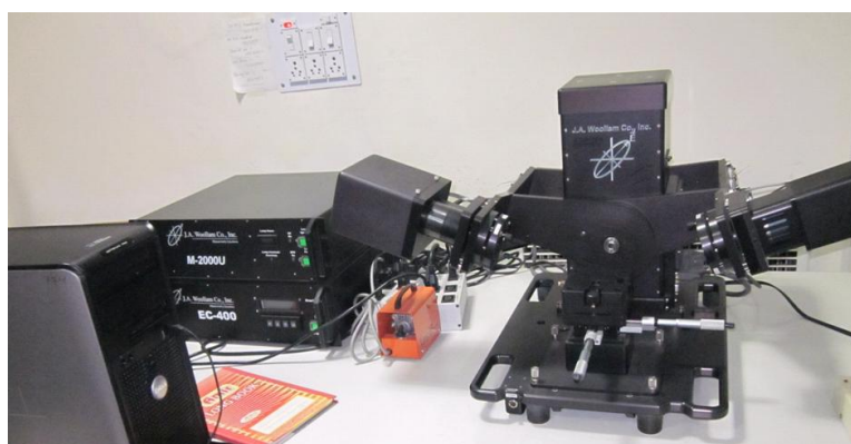
Figure 2.9: Ellipsometer used for thickness of PEDOT:PSS layer, NPL
