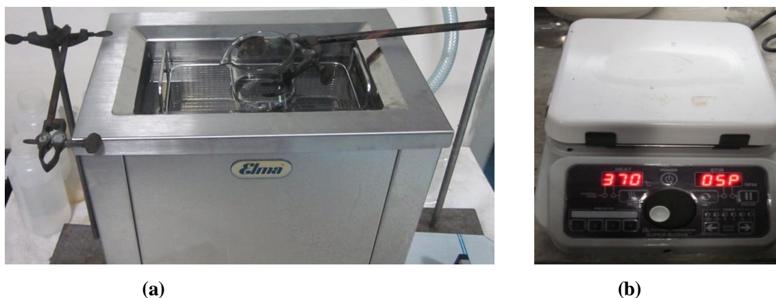
Figure 3.1(a): Sonicator with glass holder and (b) Hot plate used for ITO cleaning, at NPL .
