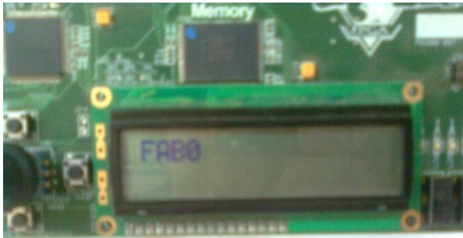
Figure6.8: LCD display (output of 16 – bit RC6 core) on Spartan3E FPGA kit
