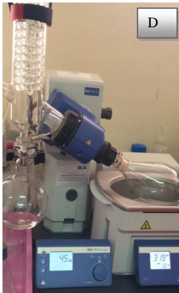
Fig 3: A) Fermented fungal cultures (1)- AS2(ii) (2)- AS1 (3)- EL (4)- AL4 B) Filtration of the fungal culture C) Solvent extraction of the filtrate D) Rota evaporator E) Fungal extracts.
