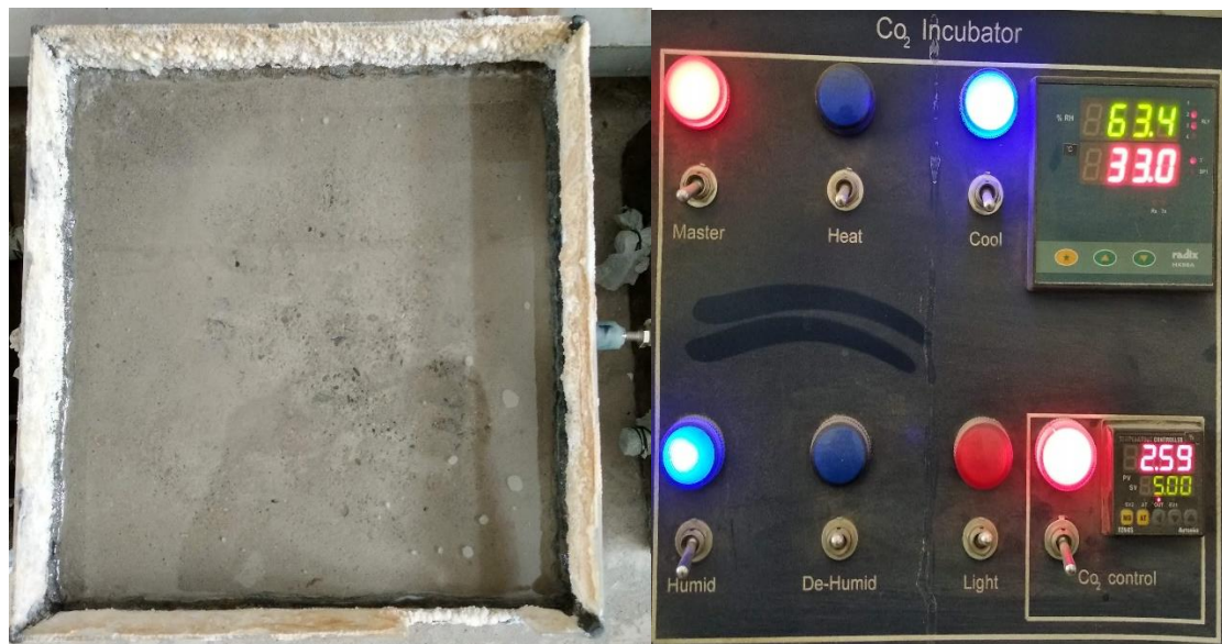
Figure 4.12 Chloride pounding on prismatic specimen (A) & CO 2 incubator (B)
