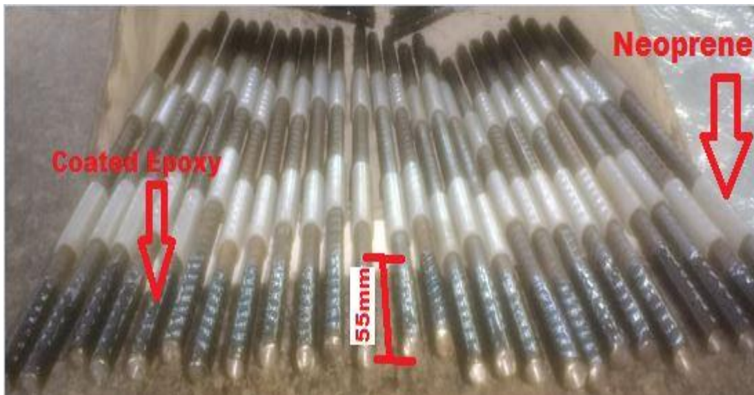
Figure 4.8 Preconditioned rebars embedded in concrete specimens
