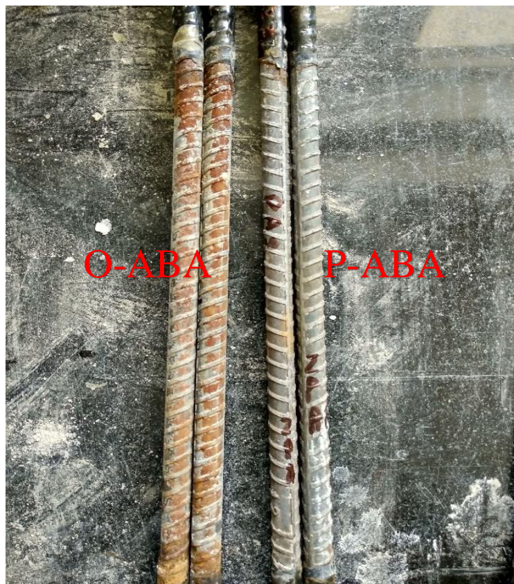
Figure 5.15 Rebars treated with 4-amino benzoic acid after completion of cycles
