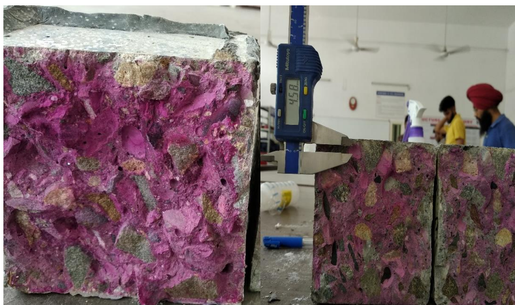
Figure 5.20 Cube after applying phenolphthalein solution (A) & Depth measurement using Vernier calliper (B)
