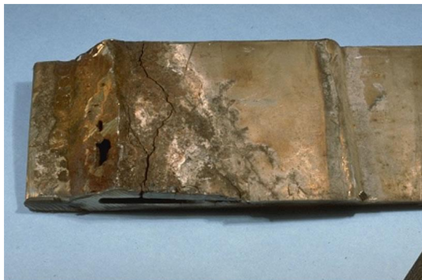
Figure 1.13 Environmental cracking corrision (Source: performancewire)
