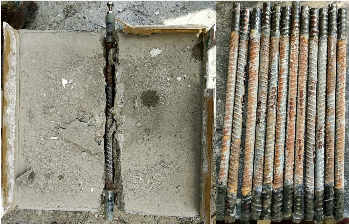
Figure 5.14 Broken Specimen (A) & All rebars collected after completion of 9 cycles (B)
