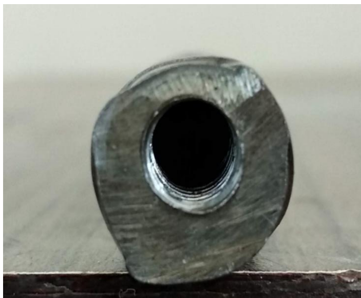
Figure 4.5 Rebar threaded from one side
