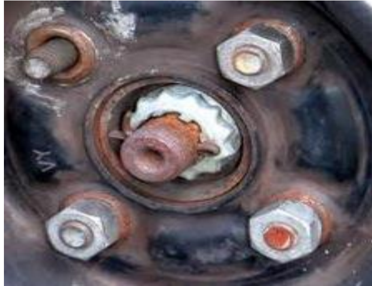
Figure 1.10 Fretting Corrosion (Source: performancewire)
