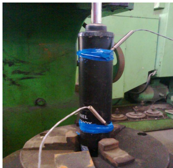
Fig. 4.1 Twin-Tube shock absorber fixed on the slotting machine for temperature measurement
