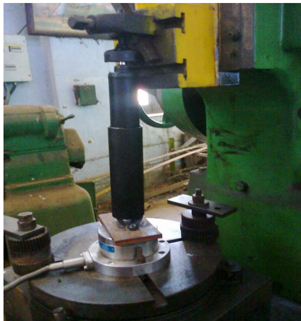
Fig. 4.2 Twin-Tube shock absorber fixed on a dynamometer for force measurement
