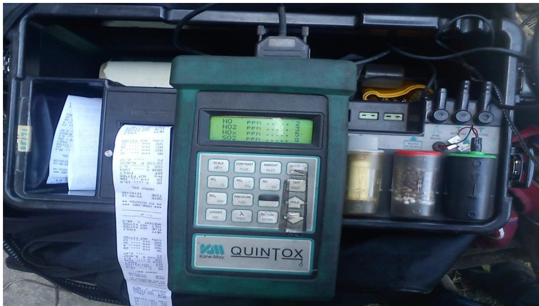
Fig 3.10 Flue gas analyzer
