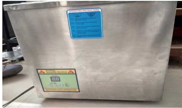
Fig 4.4 Image of Ultra-sonicator which is used for sonication of different samples.
