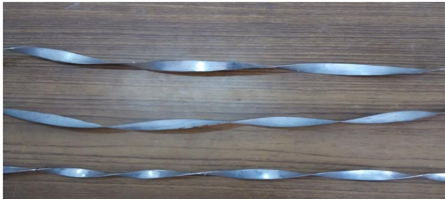
Figure 4.10 Twisted tape inserts
