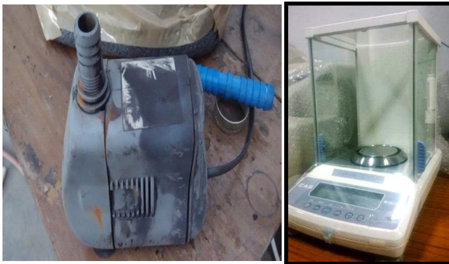
Figure 4.12 Pump used in hot tank and weighing machine for measuring the weight of nanoparticles.
