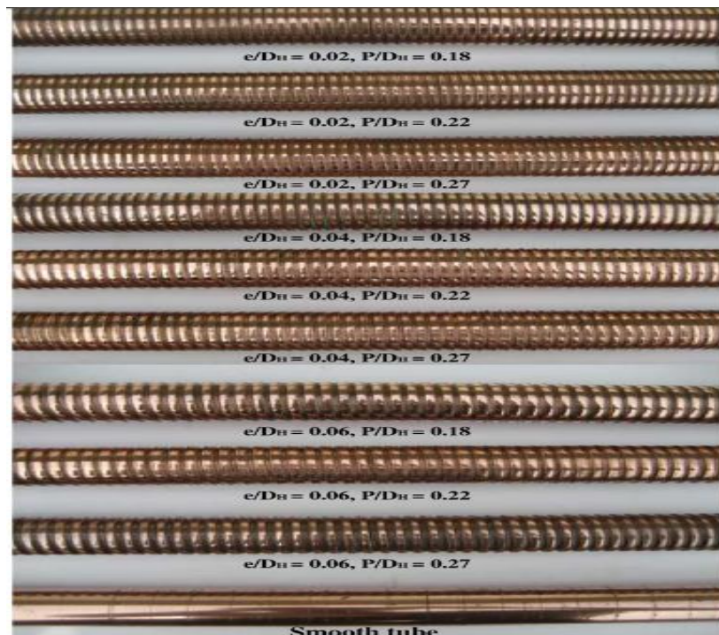
Figure 8.8 Tubes with different twist ratio and rib ratio
