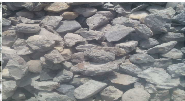
Figure 1.4 Presoaked recycled aggregates
