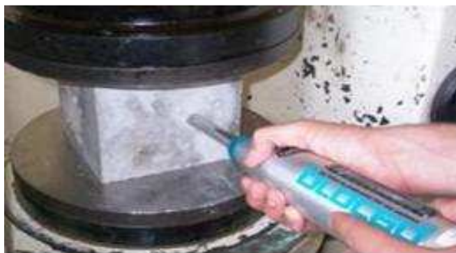
Figure 3.17 Rebound Hammer Test for Specimen
