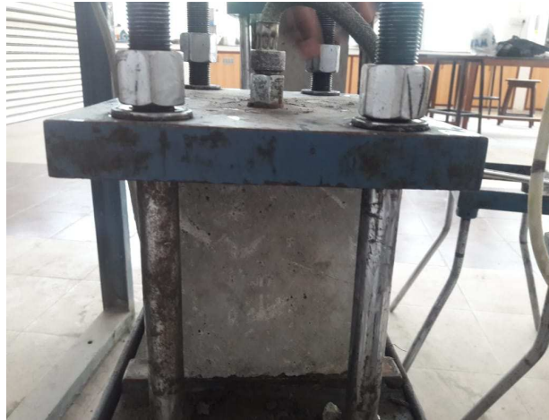
Figure 3.20 Water Permeability Test
