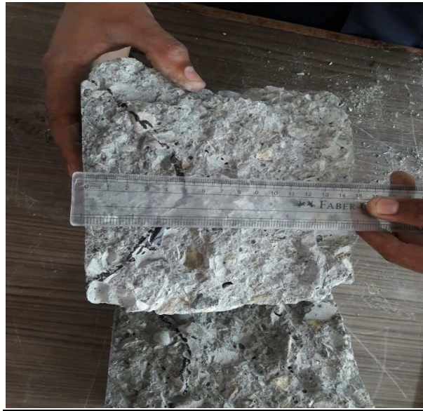
Figure 3.22 Water Permeability Depth
