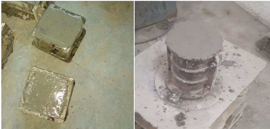
Figure 3.9 Moulds filled by Concrete
