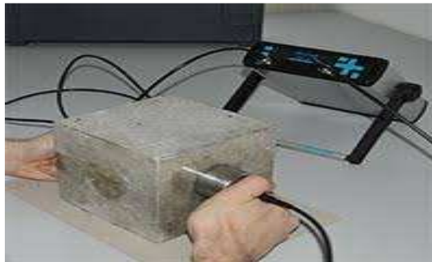
Figure 3.15. UPV Test of Concrete Cube
