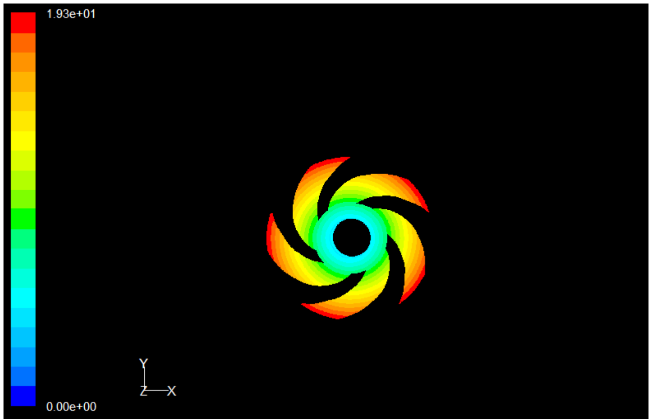
Figure 5.3: velocity contours at impeller (Q= 0.0 lps, N= 1400 rpm)
