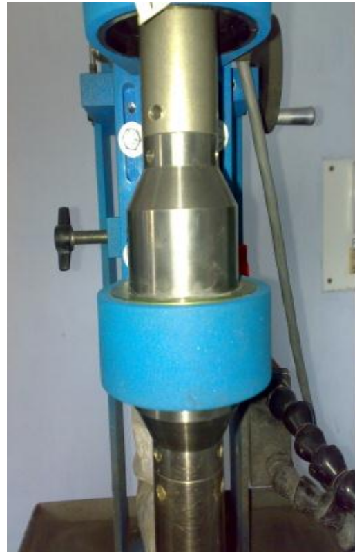
Fig:7.3 Amplitude coupling for compact 500W Ultrasonic Machine
