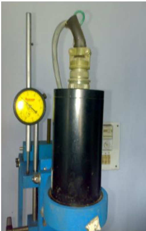
Fig:7.4 Ultrasonic Transducer for Compact 500W Ultrasonic Machine
