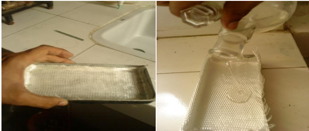
Fig 4.10 Pouring of EPDM/Clay mixture on Glass Fibre Sheet
