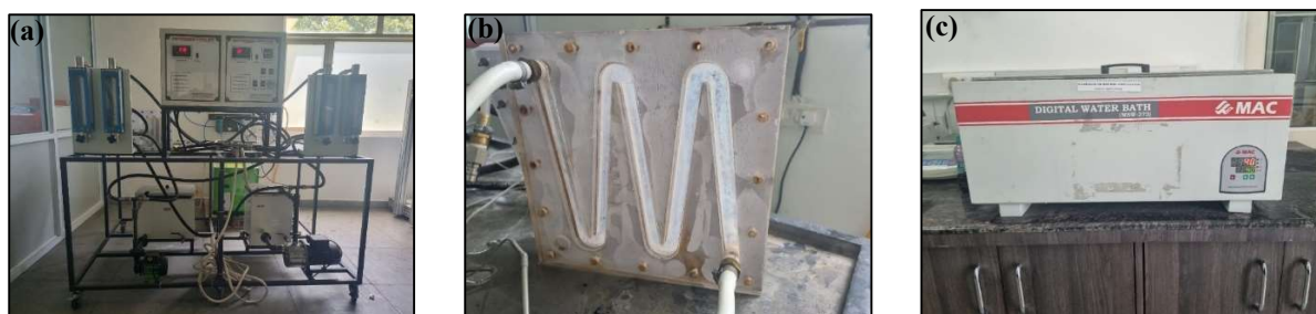
Fig. 3.2 shows (a) heat exchanger test rig (b) acrylic sheet (c) water bath
