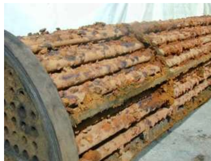
Fig. 1.5 Corrosion on Heat Exchanger
