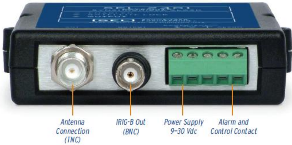
Figure 37: SEL-2401 Functional Overview Bottom [33]
