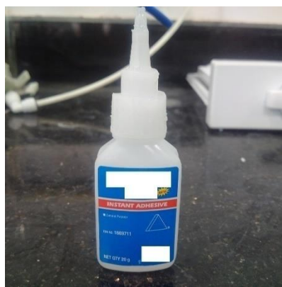
Fig. 5.14 Instant adhesive used for joining HIPS and 3D printed screws
