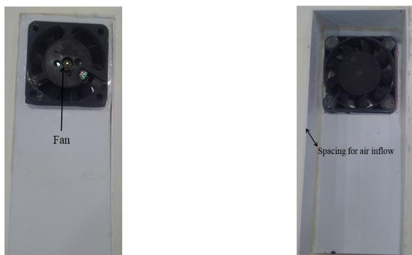
Fig. 5.4 Duct with fan
