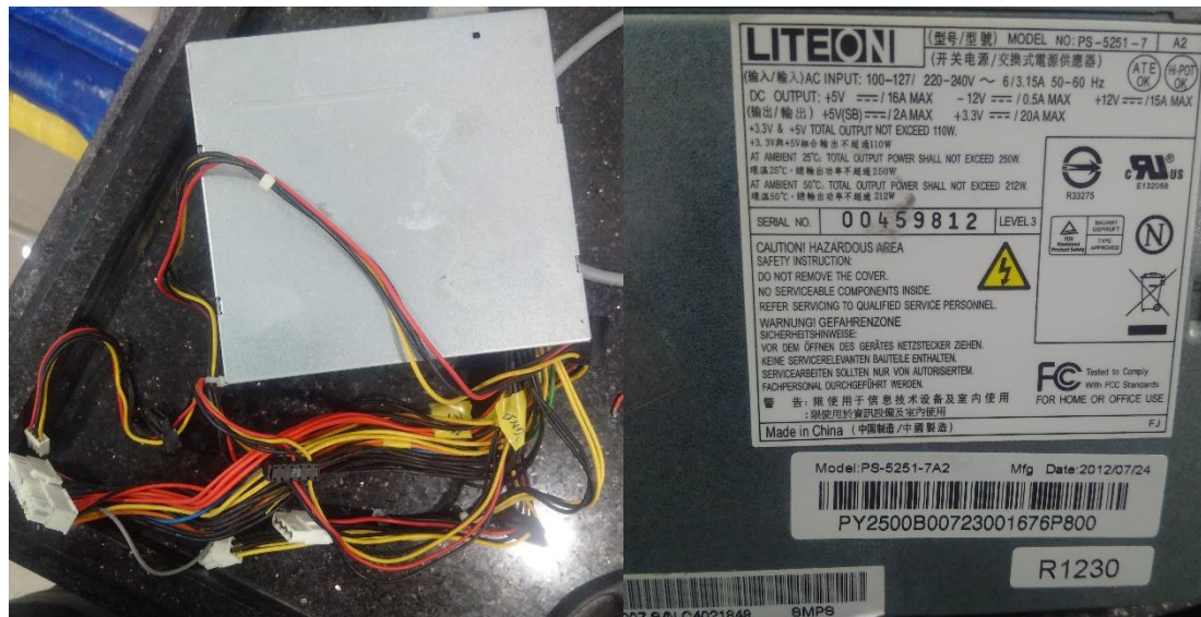
Fig. 5.8 PC power supply and its specification
