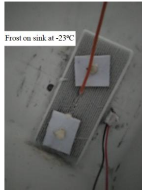
Fig. 5.21 Frost deposited on the sink
