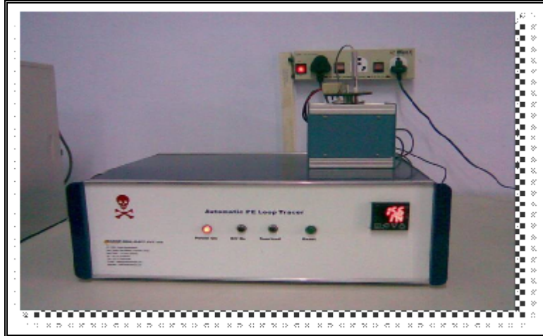
Figure 2.10. Experimental setup for ferroelectric hysteresis measurement system
