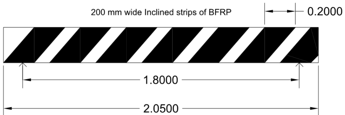
Figure 3.11 Details of Beam Strengthened with Arrangement-III
