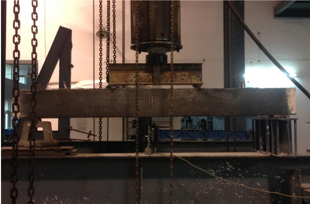
Figure 3.10 Test Setup for Beam Strengthened with Arrangement-II
