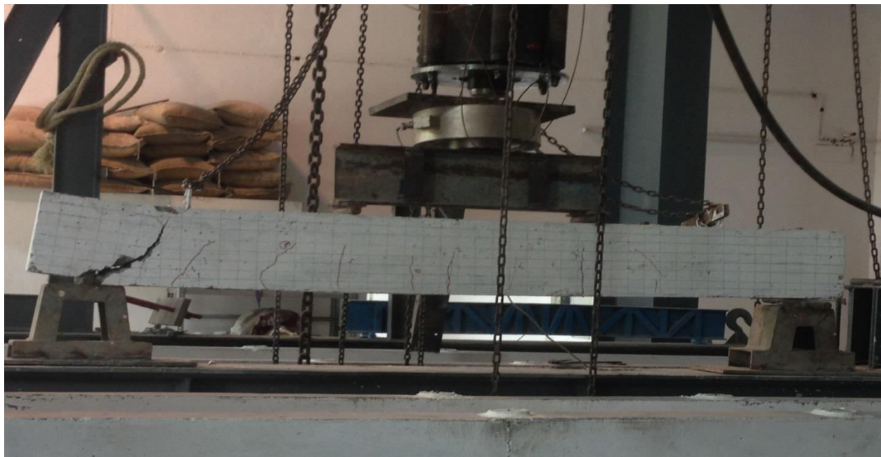
Figure 4.3 Failure and Crack Pattern in Referenced Beam
