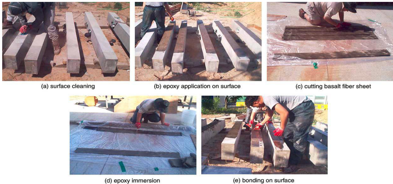
Figure 2.8 Strengthening procedure for basalt fiber sheet [Sim et al., (2005)]
