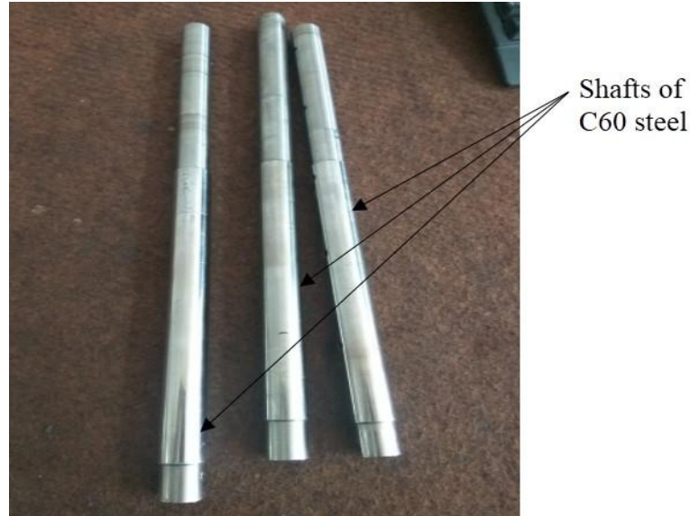
Figure 2.4: Grounded shafts of steel of grade C60 used for experimentation
