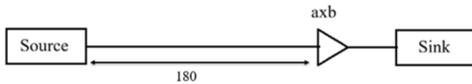
Fig 7.3: Single-Buffer Path with Long Signal Propagation Distance
