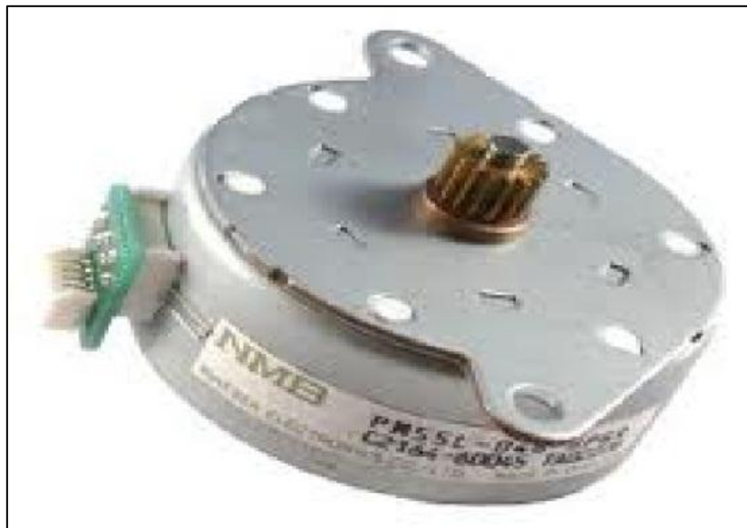
Figure 3.1: Stepper motor used for test hardware
