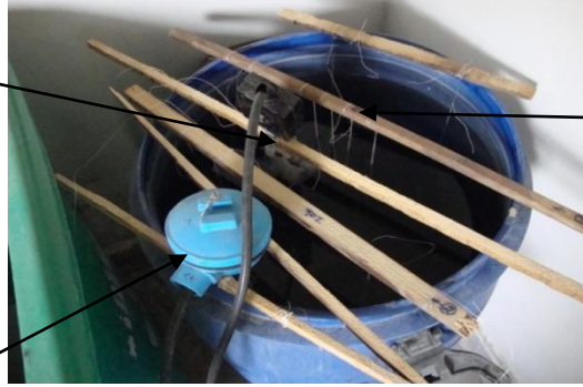
Fig. 4.17 Heating Element and RTD sensor in a tank
