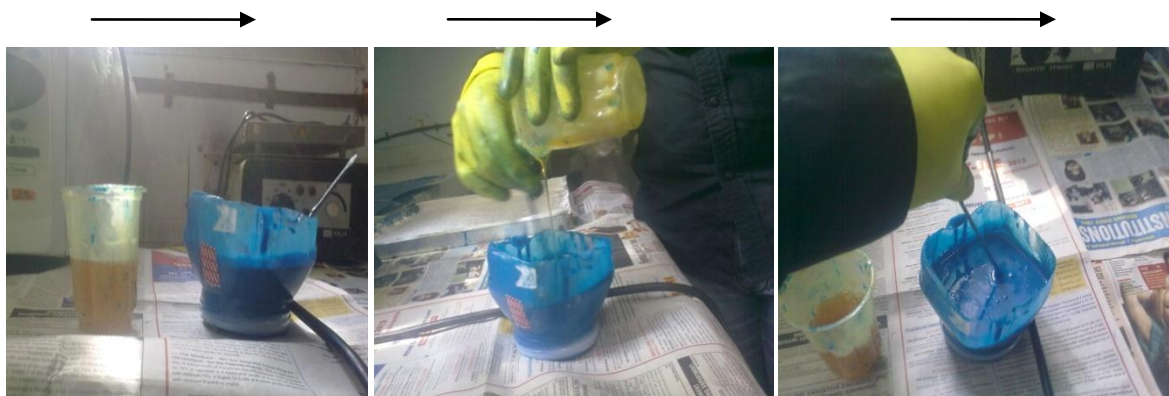
Fig. 4.9 mixing of hardener to the base component
