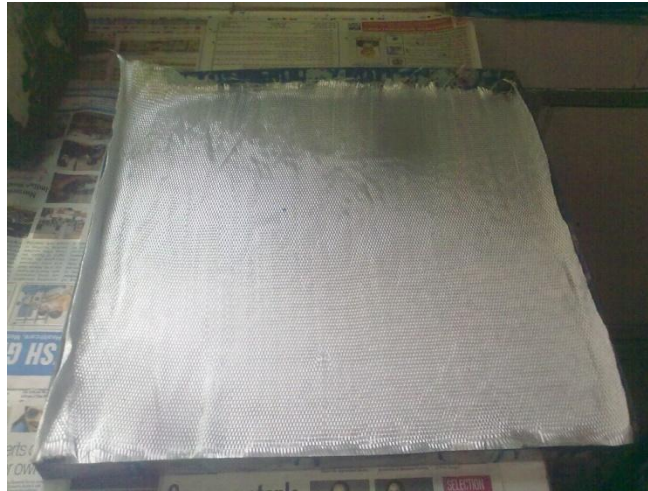
Fig. 4.6 Uncoated glass fibre mat used for making specimen
