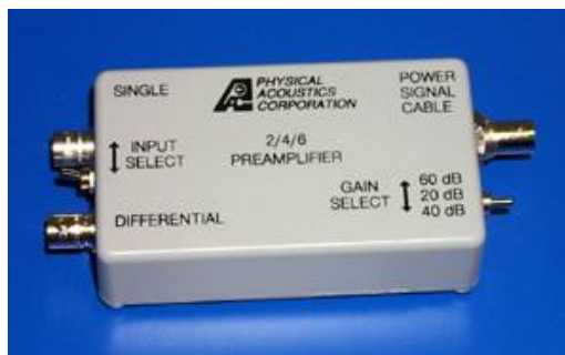
Fig. 5.8 Preamplifier used in the study
