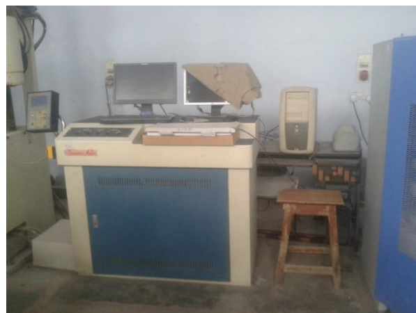
Fig. 5.10 Setup used to operate UTM with computer
