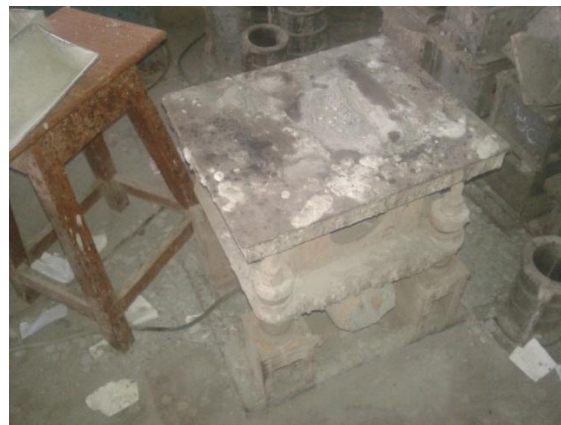
Fig. 5.3 Vibrating table used for setting concrete
