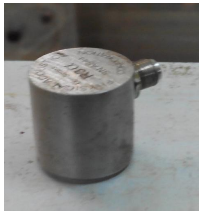
Fig. 5.7 R3 \alpha sensor used in present study
