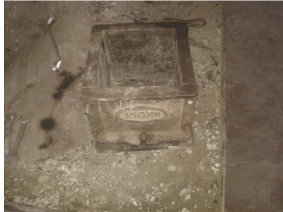
Fig. 5.2 Casing used for casting concrete cubes
