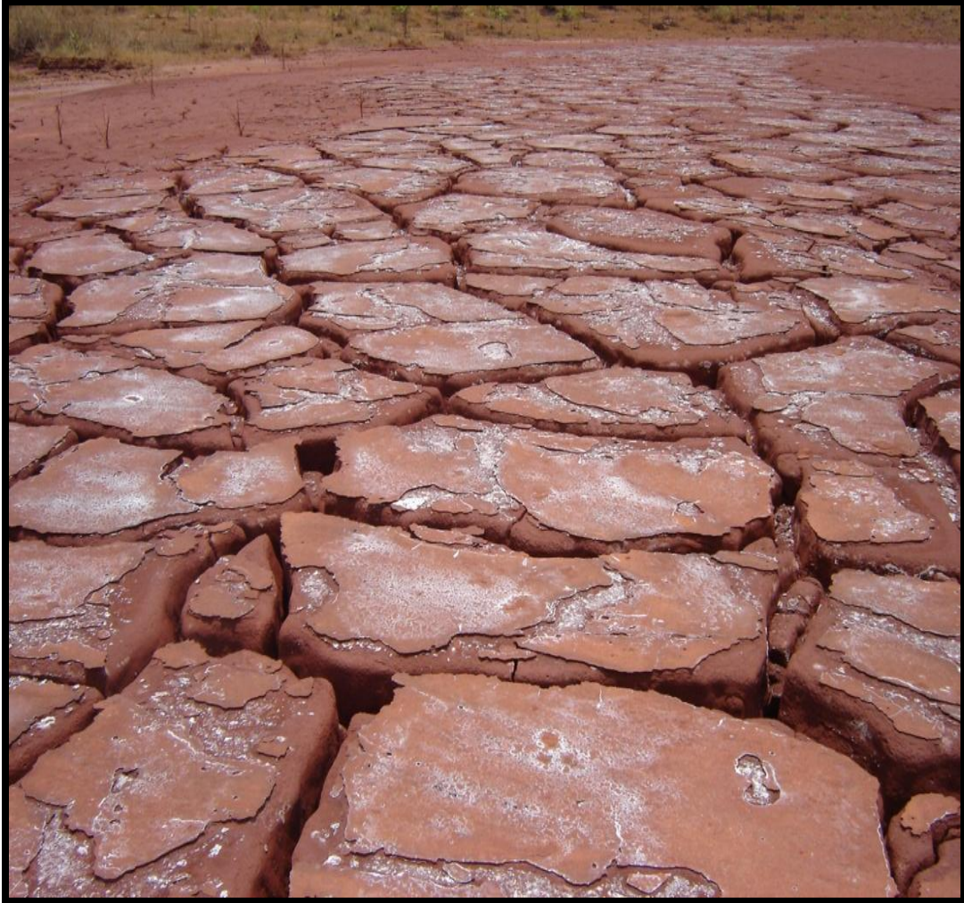
Fig 2.1: Deposition of soda flakes, which appears white on the surface of red mud pond at NALCO, Damanjodi, Orissa, India.
