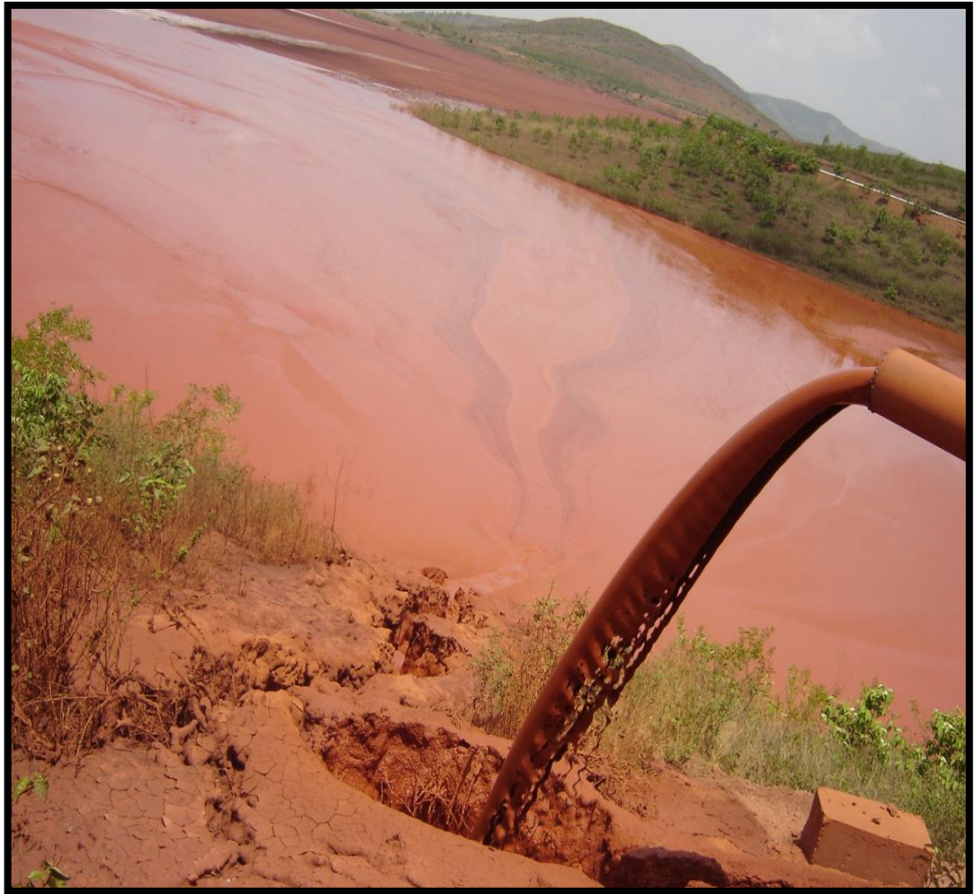
Fig 1.2: Disposal of red mud in the form of wet slurry to nearby artificial impoundments at NALCO, Damanjodi, Orissa, India.
