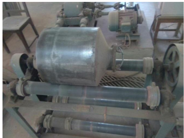
Figure 4.1: Pictures of dry ball mill (make AS Enterprise, Calcutta)
