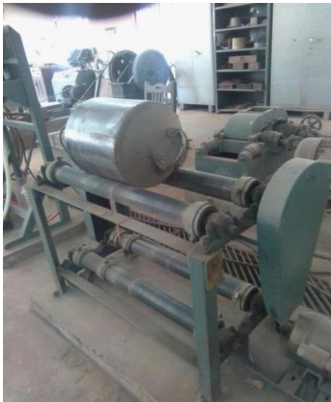
Figure 4.1: Pictures of dry ball mill (make AS Enterprise, Calcutta)
