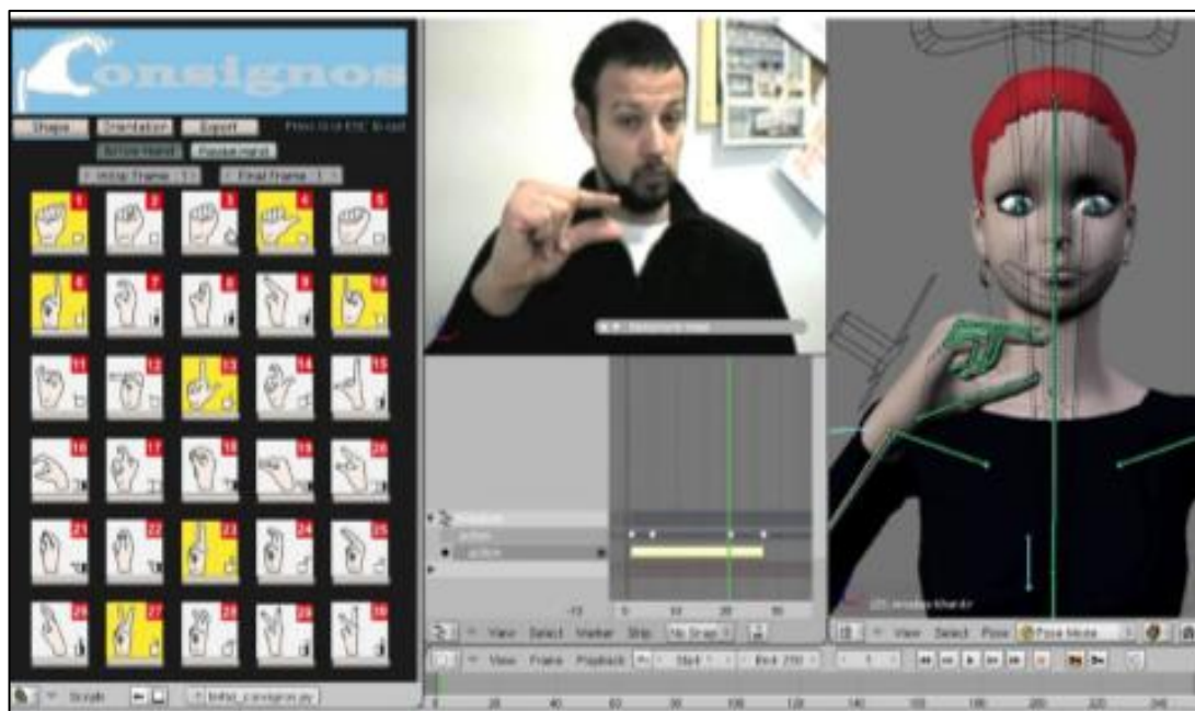
Figure 2.14. Sign editor based on the use of predefined static poses for hand shape and orientations [32]
