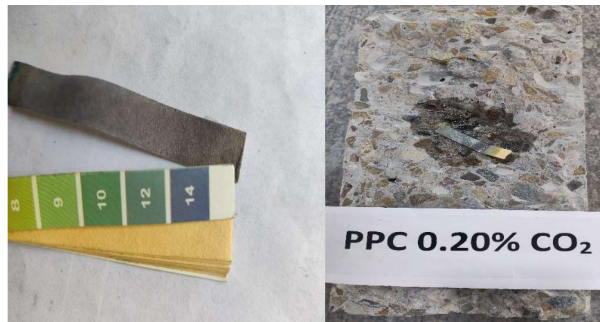
Figure 4. 26 pH paper test results for all mixes
