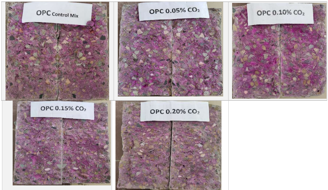
Figure 4. 29 Phenolphthalein sprayed specimens at 56 days (OPC based mixes)
