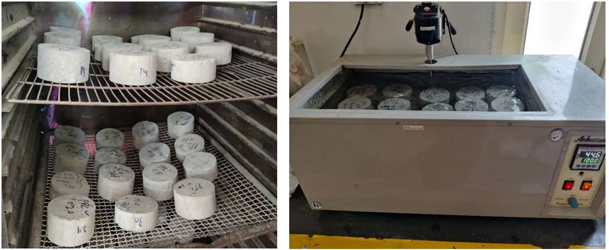
Figure 3. 17 Water absorption test: oven drying of samples (left) and immersion in boiling water (right)
