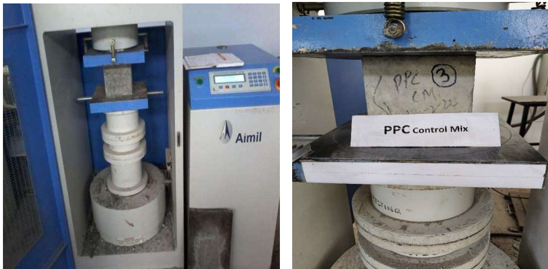
Figure 3. 13 Testing of specimen for compression in CTM
