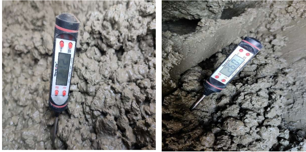
Figure 3. 9 Temperature of the concrete
