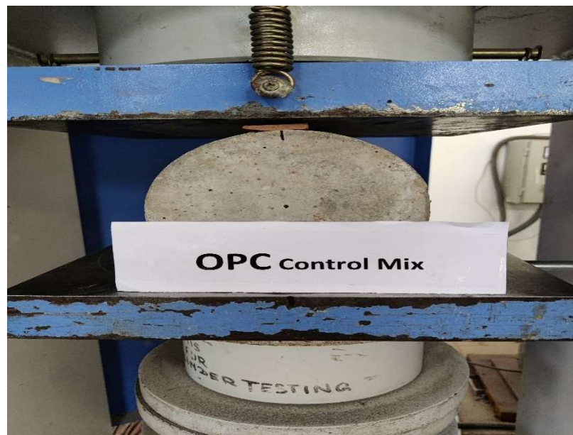
Figure 3. 14 Testing of specimen for split tensile strength in CTM
