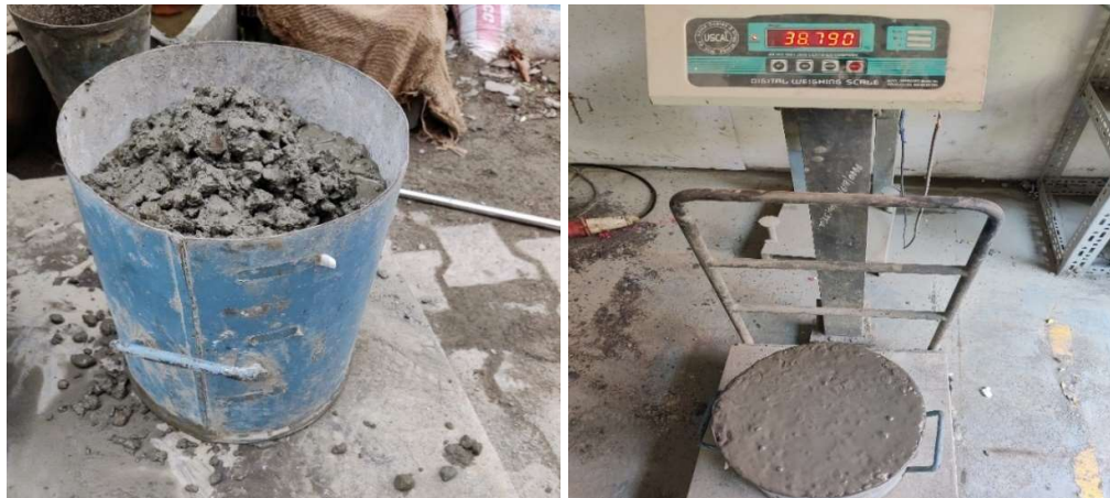
Figure 3. 10 Density of the concrete measurement
