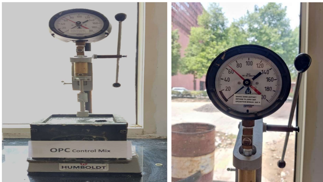
Figure 3. 11 Test apparatus for determining the setting time of the concrete
