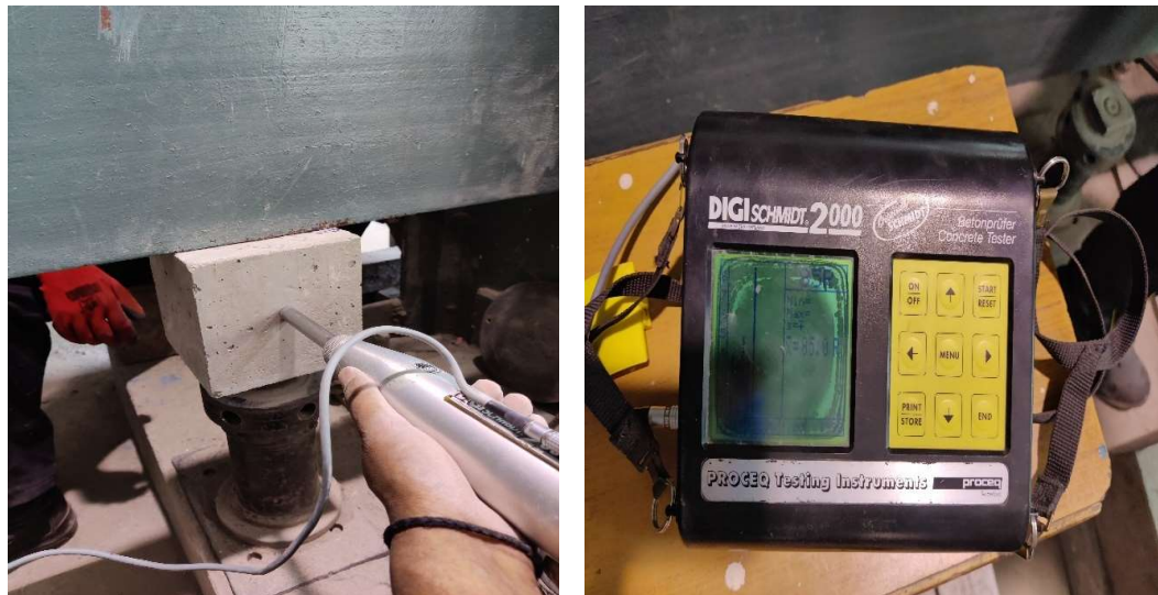
Figure 3.19 Performing the rebound hammer test on concrete specimen
