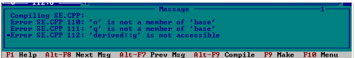
Figure 5.3 Variable of derived class is not class not accessible by base class Screen shots of simple inheritance of variable accessibility with an object are shown in figure 5.4. Similarly is the case in which accessibility of variable with different functions. Its screen shots are shown are shown in figure 5.5
