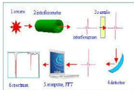
Fig. 4.8 Block diagram of FTIR [25]
