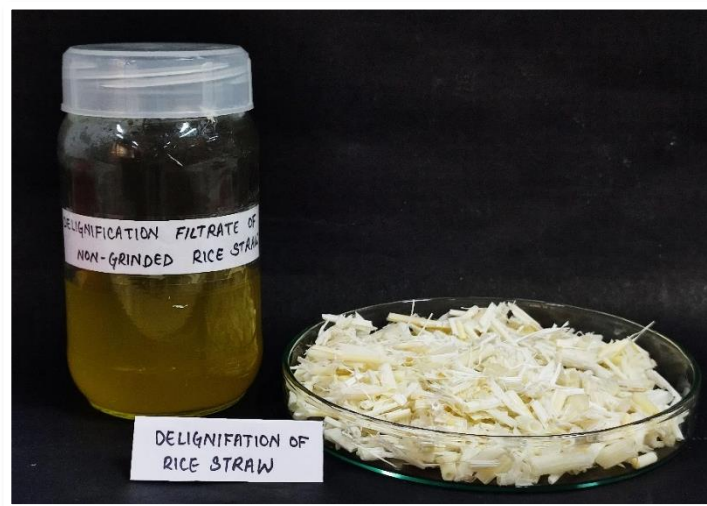
Figure 7: Rice straw after acid treatment process (delignification)
