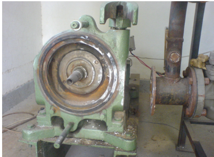
Figure 5.1 Disassembled view of centrifugal slurry pump
