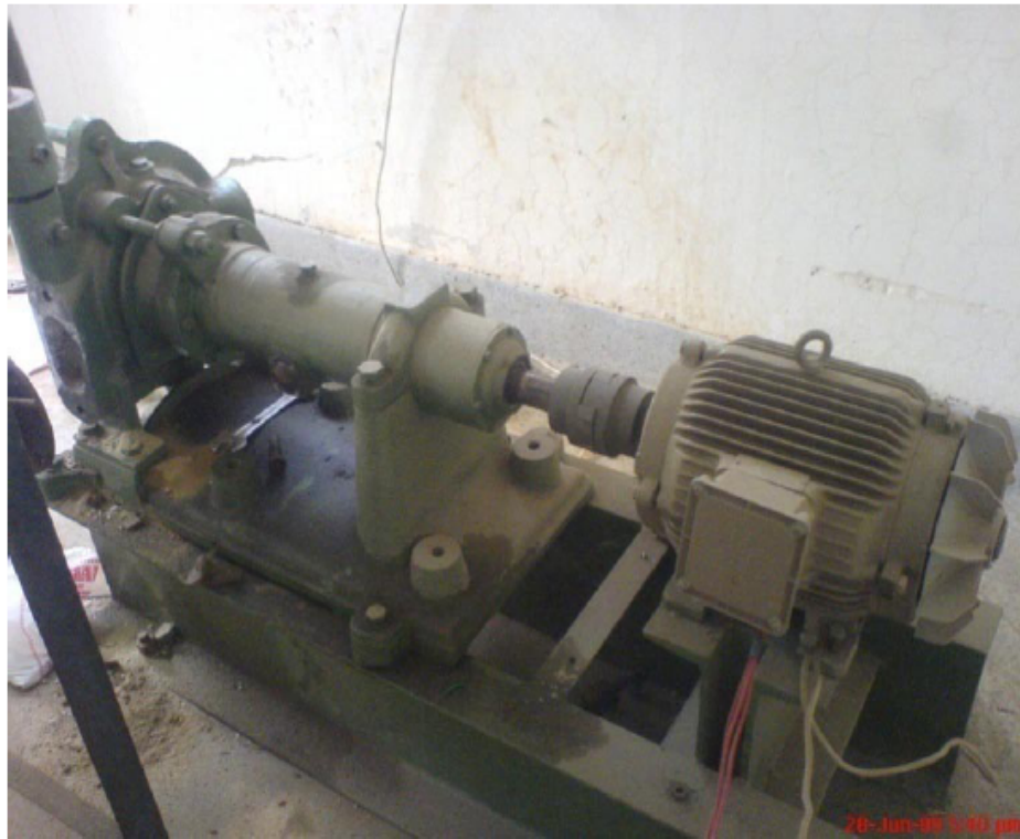
Figure 3.6 Centrifugal slurry pump of the test loop
