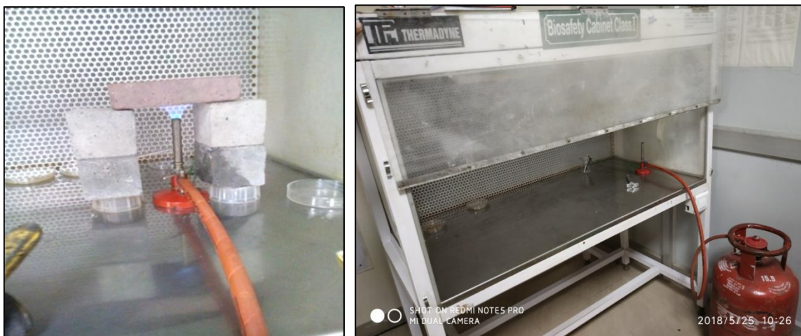
Fig 3.16 Bunsen Burner setup and testing of Sample
