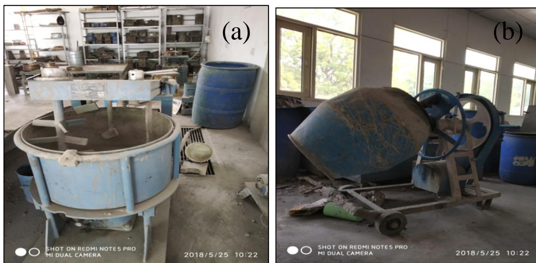
Fig 3.7 Pan mixer (a) and the concrete mixer (b) used for mixing the concrete constituents
