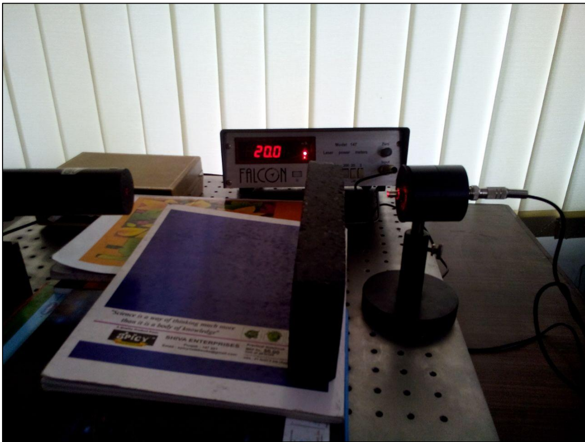
Fig 3.10 Transmission testing setup with an optical power meter
