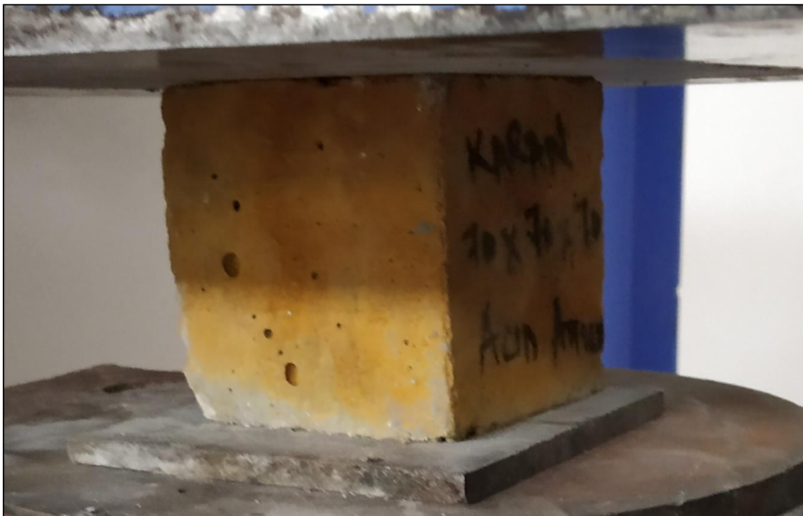
Fig 4.12 Sample with eroded surface and yellowish stains due to acid
