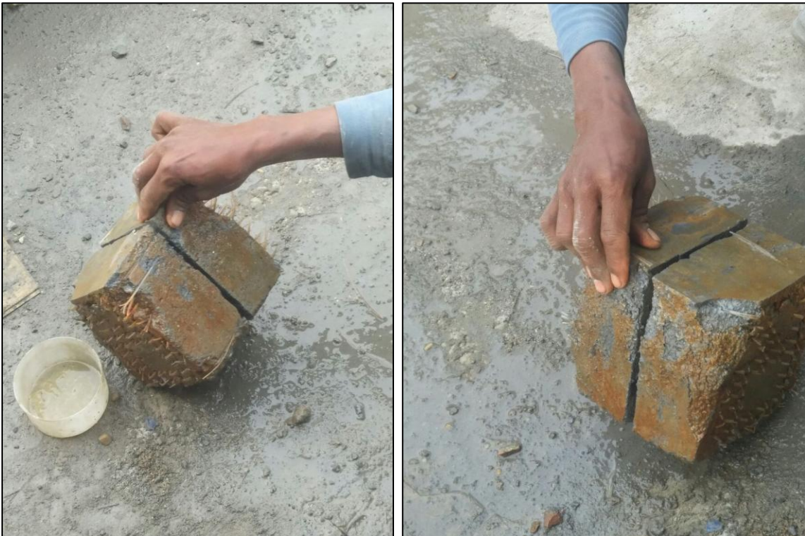
Fig 3.13 Concrete Block Sample with a Clear cut from the middle
