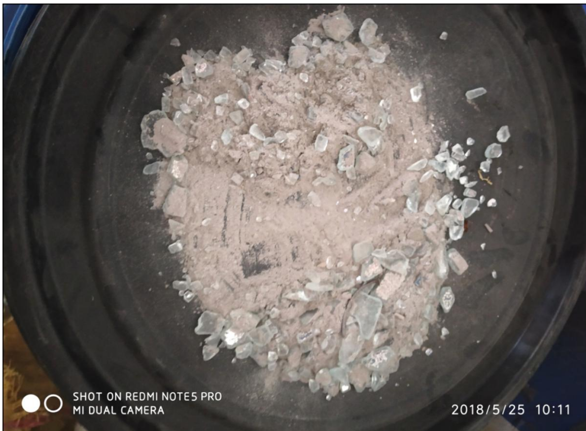
Fig 3.3 Waste Glass Aggregates after crushing by L.A Abrasion Machine
