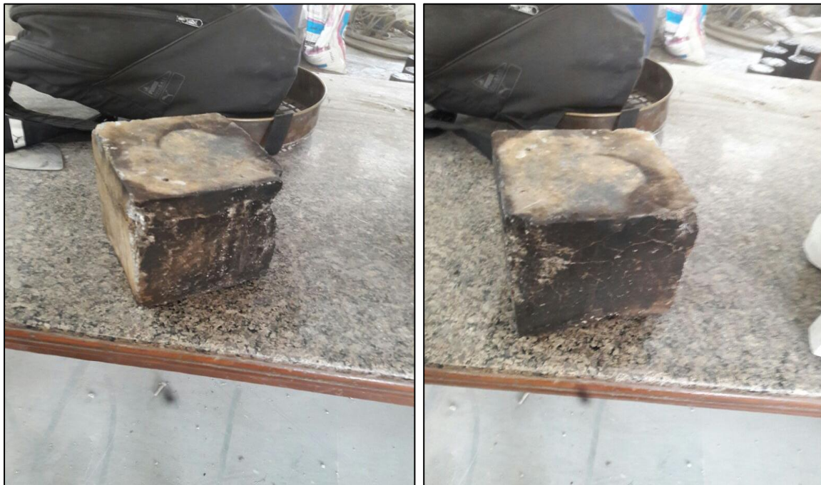
Fig 3.15 Flash Fire test of Sample for Transmission test
