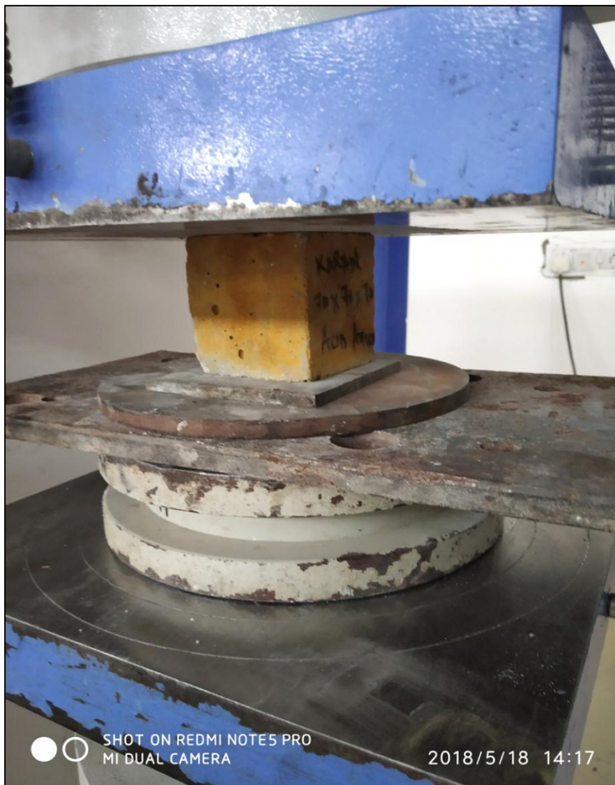
Fig 3.14 Compression testing of Sulfuric attacked sample
