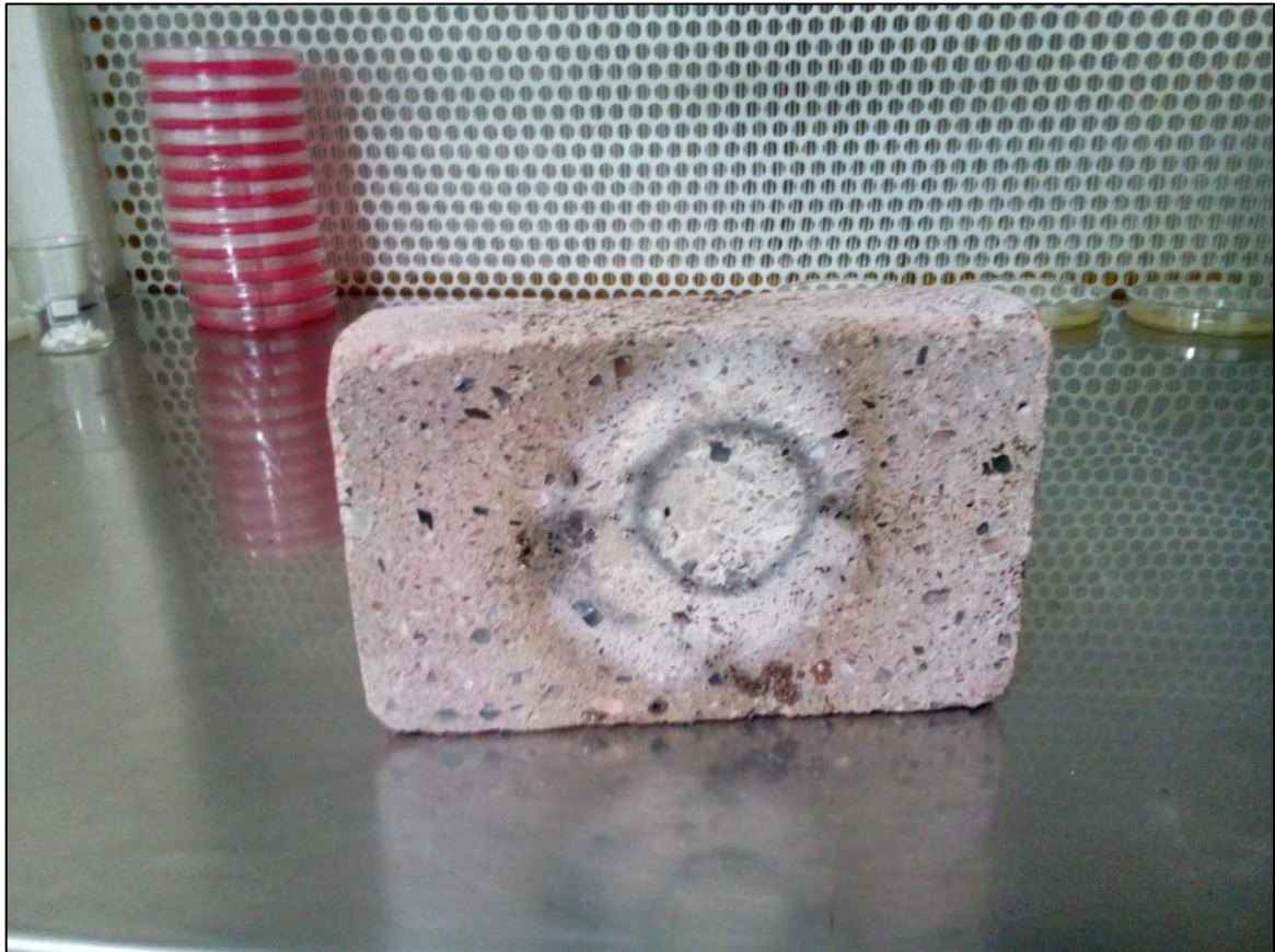
Fig 4.13 Sample after one-hour fire test
