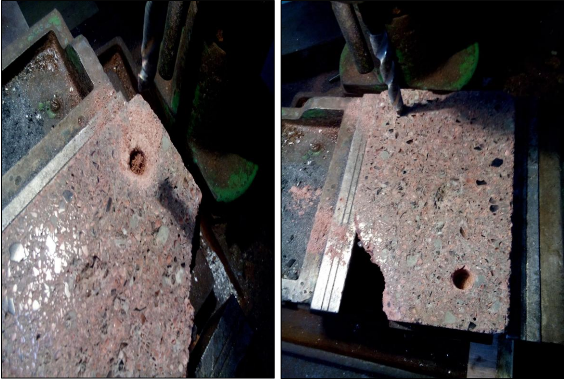
Fig 3. 12 Subsequent drilling of the Sample at near edge in cross section
