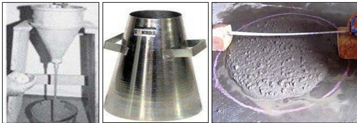
Fig 3.9 Equipments for slump flow test
