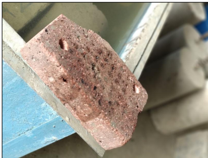
Fig 4.18 Sample after oil spill test
