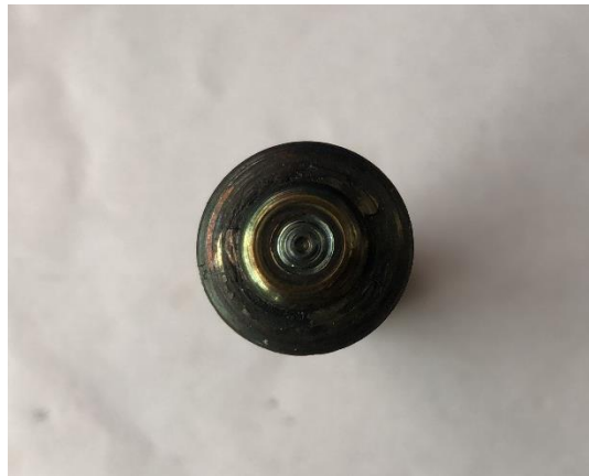
Fig 5.19 Distorted tool pin
