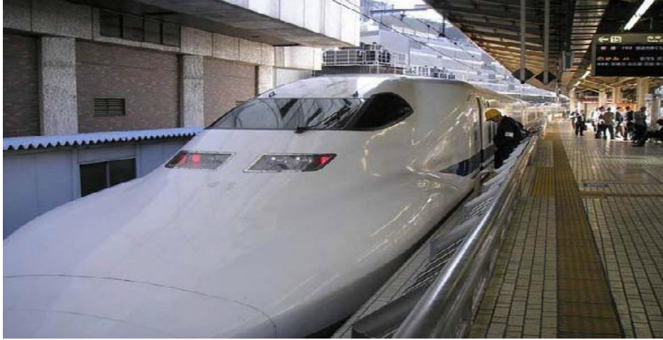
Fig 1.7 Japanese railway rolling stock fabricated from aluminum by FSW (Rowe and Thomas, 2006)
