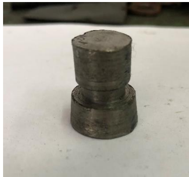
Fig 4.11 Tool support that transmits load to spindle
