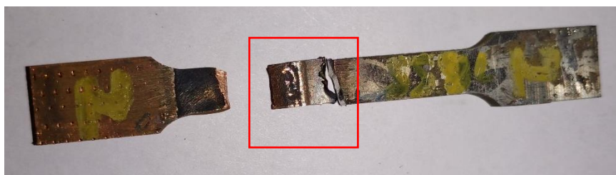
Fig 7.7 Sample extraction for fractography (SEM)
