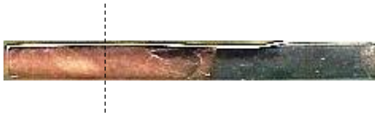
Fig 7.16 TMAZ Cu-Cr-Zr (Ultimate tensile break point)
