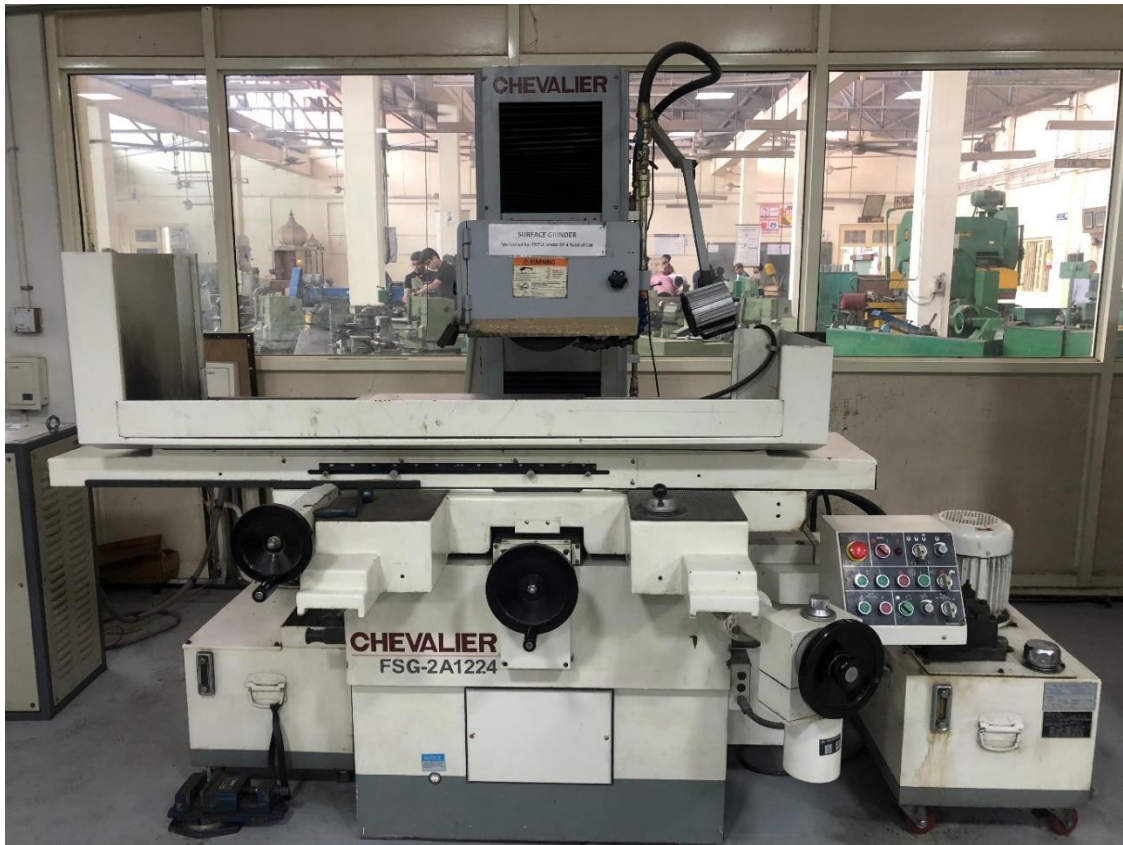
Fig 6.10 Surface grinder with magnetic chuck
