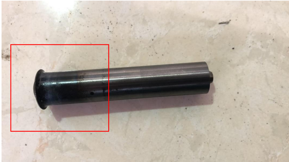
Fig 5.18 deformation in tool due to heavy heat and force produced
