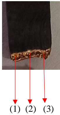
Fig 7.8 Top, intermediate and bottom points in TMAZ (Cu-Cr-Zr) for fractography
