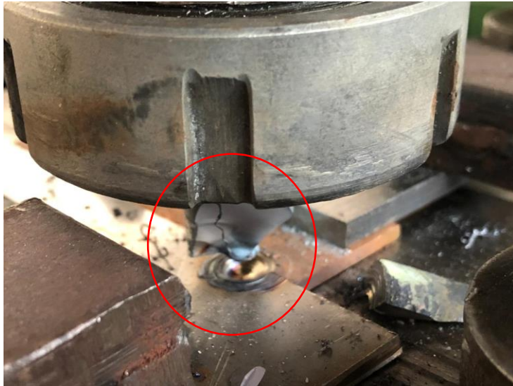
Fig 5.13 Tool crack due to impact force
