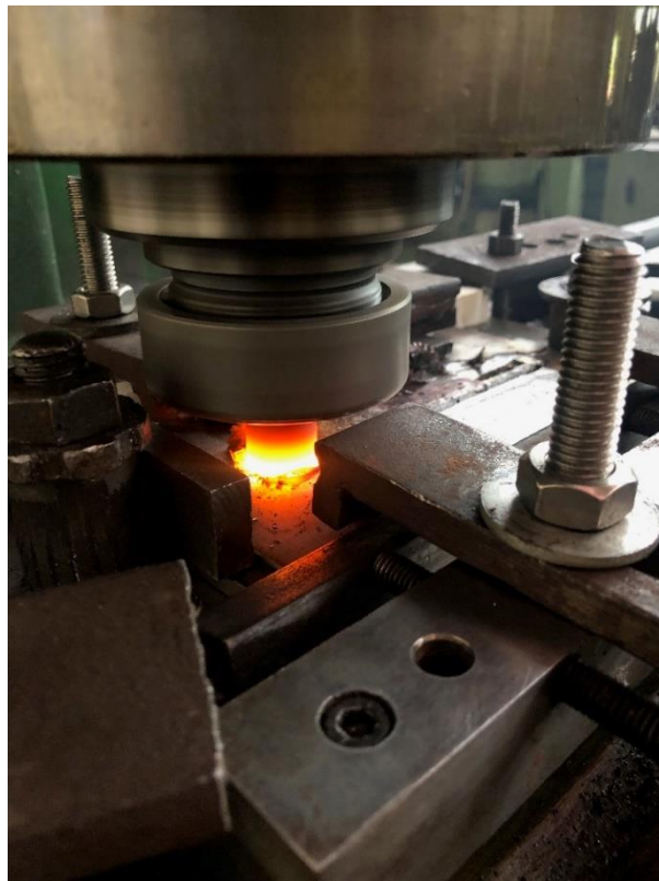
Fig 5.9 Friction stir welding of SS 304/Cu-Cr-Zr at 2 degree of tilt angle
