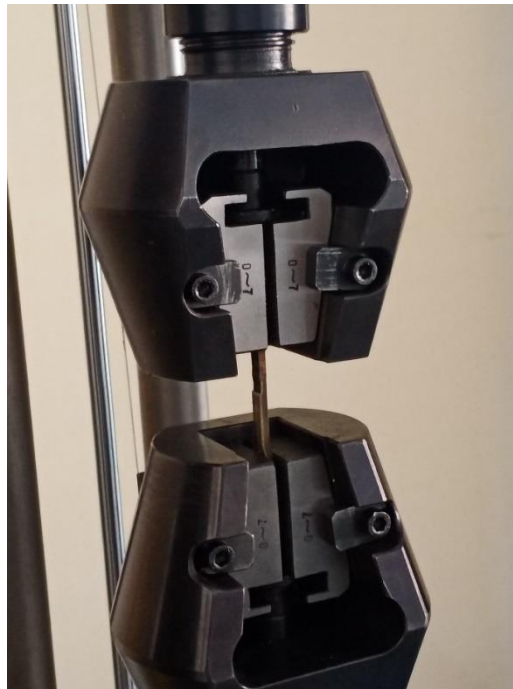
Fig 6.4 Cross weld tensile testing
