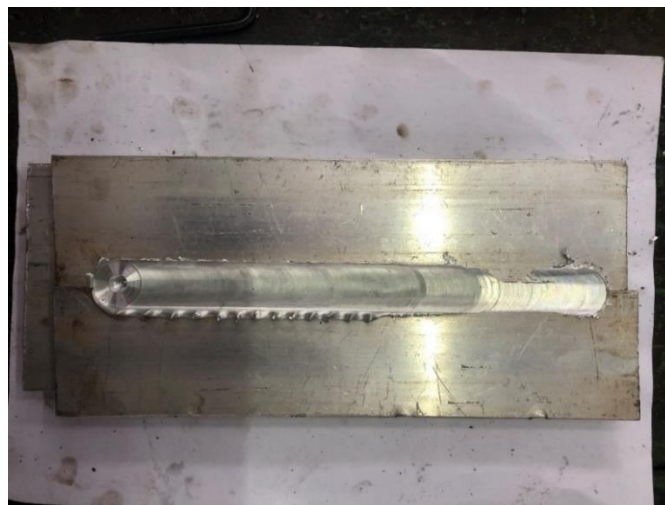
Fig 4.13 Backing plate weld with work piece
