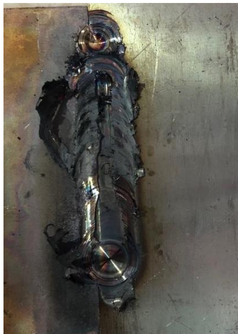
Fig 5.10 Defect in welding at 900 rpm
