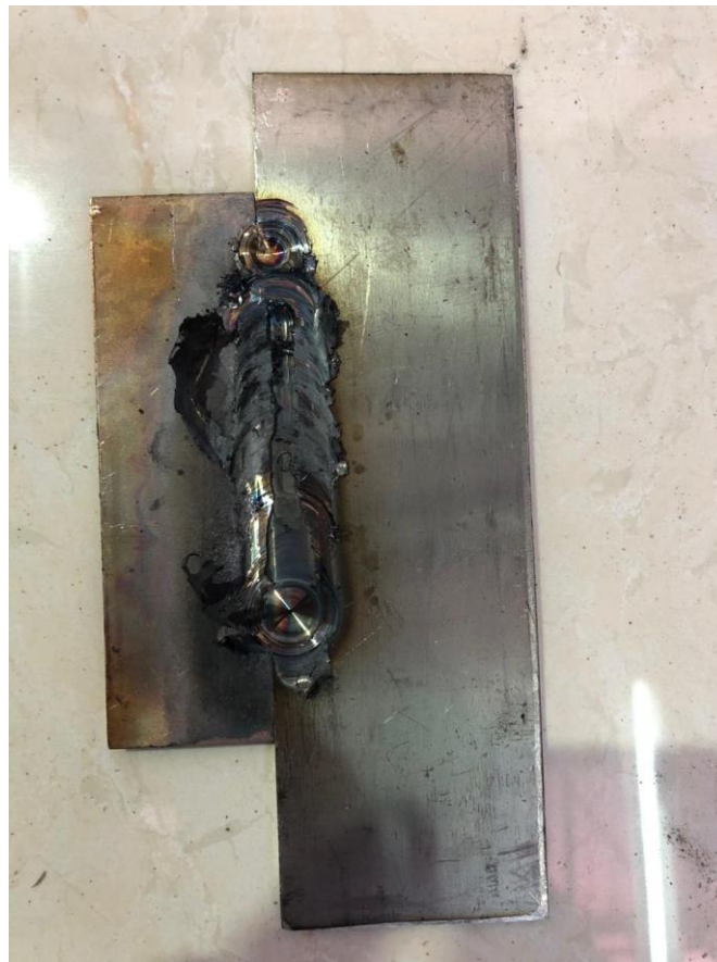
Fig 5.11 Defect in welding at 1200rpm
