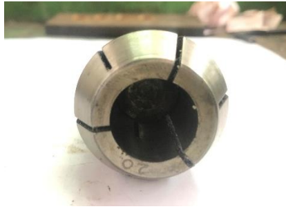
Fig 4.10 Gap remain in collet after tool insertion
