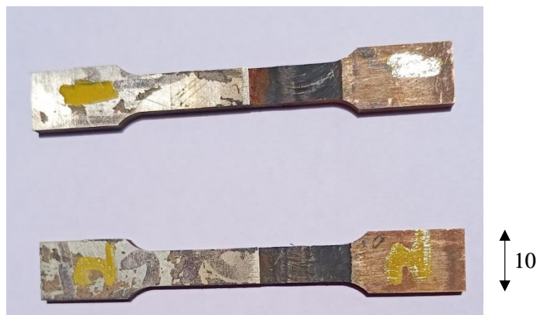
Fig 6.18 Cross weld tensile testing specimen
