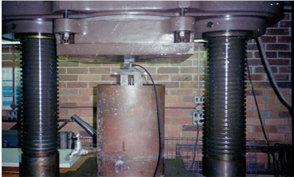
Figure 2.9 Apparatus for Expansion force test(Wang, 2010)
