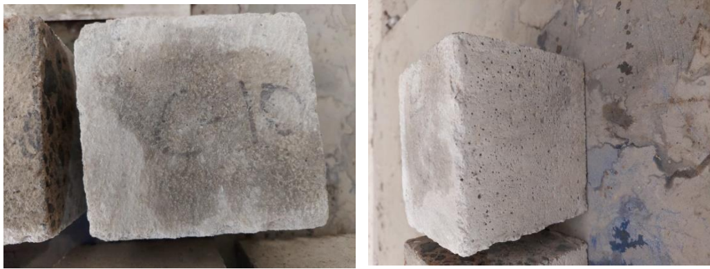
Figure 4.37 Hot water curing
