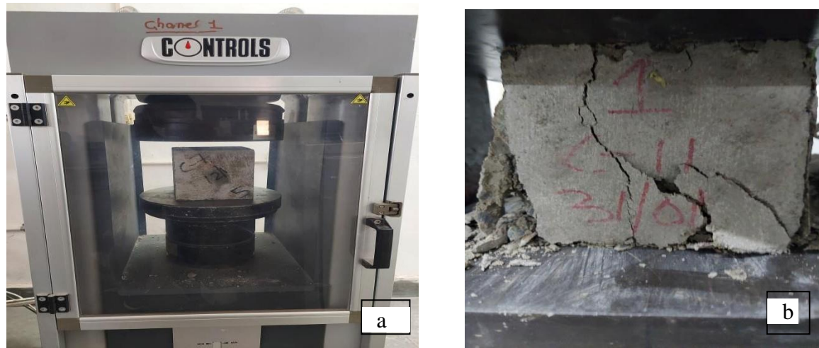
Figure 4.5 Compressive strength testing of cube
