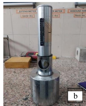
Figure 4.26 (a) Rebound hammer testing on cube (b) Schmidt rebound hammer
