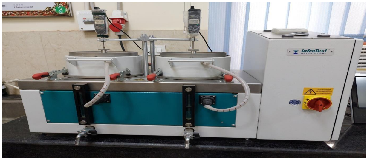
Figure 3.11 Steam exposure device
