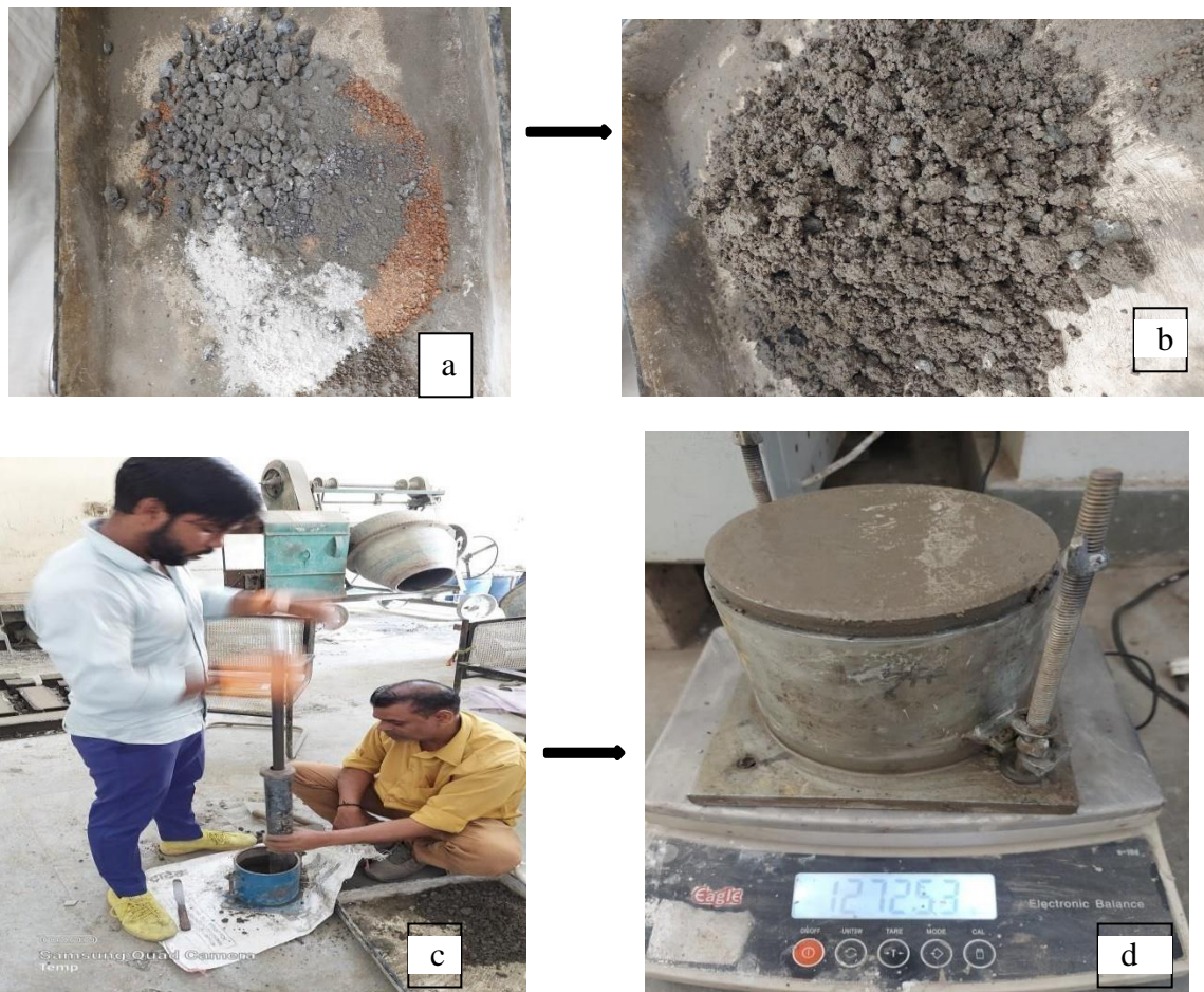
Figure 3.37 Modified Proctor Test
