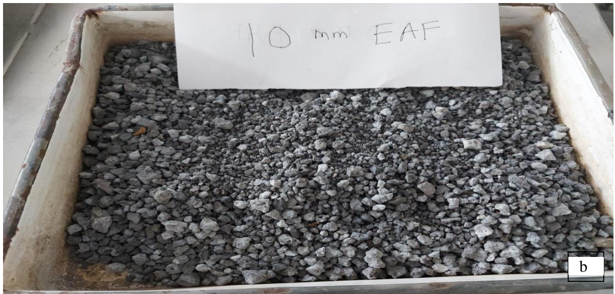
Figure 3.6 (a) 20mm EAF slag aggregate after stabilization (b) 10mm EAF slag aggregate after stabilization
