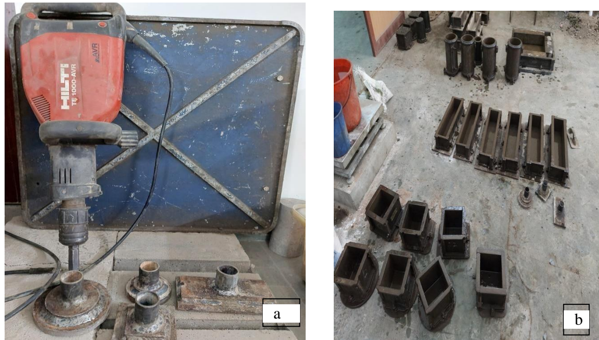
Figure 3.38 (a) Plates used in compaction (b) Moulds casted
