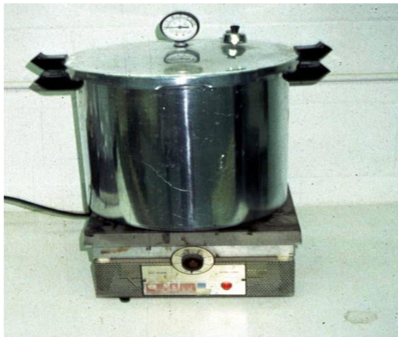
Figure 2.10 Apparatus for Disruption Test (Wang, 2010)
