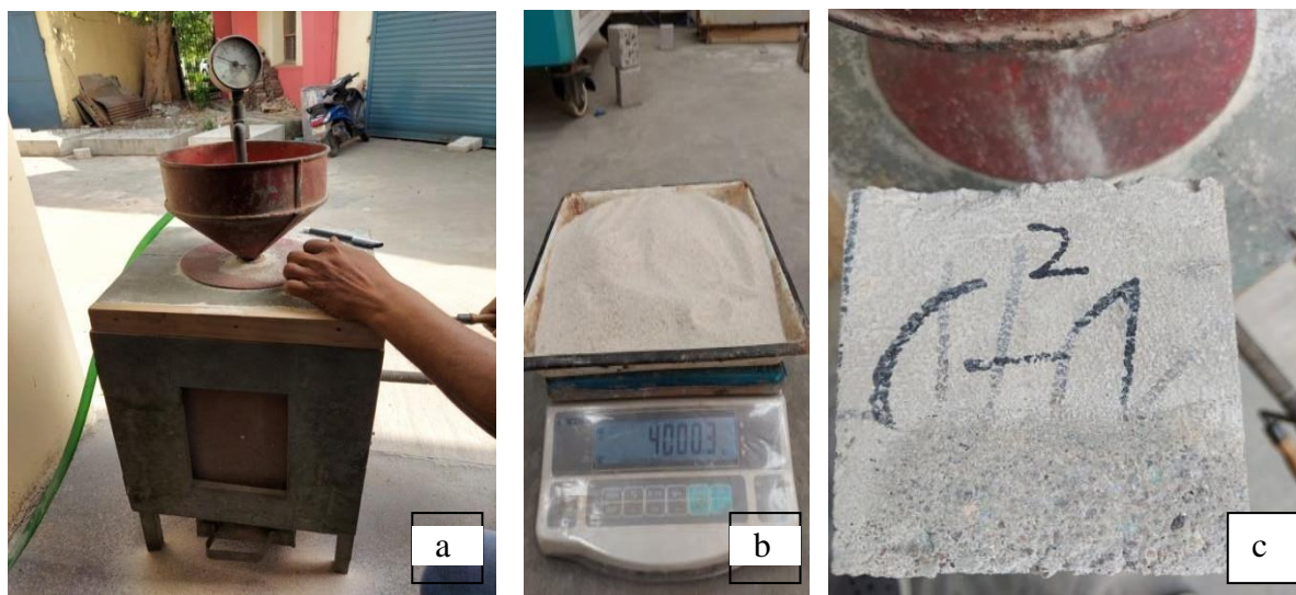
Figure 4.29 (a) Sand blasting machine ,(b) Ennore sand used ,(c) After abrasion of 1 st surface of E00 mix
