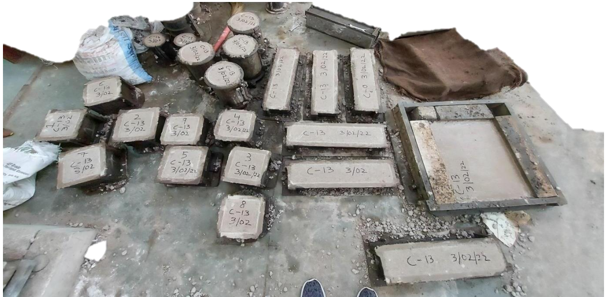
Figure 3.41 Casting after 24 hours of E50G50 mix before demoulding
