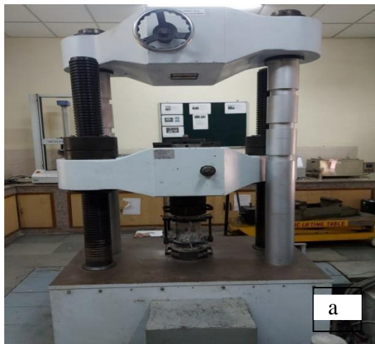
Figure 4.22 Testing for modulus of elasticity on cylinder
