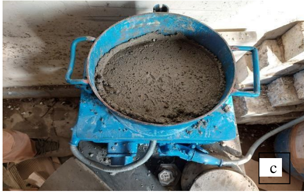
Figure 4.3 (a) Vebe apparatus, (b) Modified vebe test ,(c) Completion of modified vebe test
