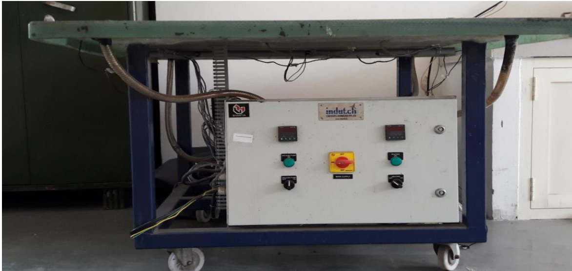
Figure 1.12 : Vacuum assisted resin infusion molding machine with on mould heating system (Photo courtesy: Chemical Engineering Department, Thapar University, Patiala)
