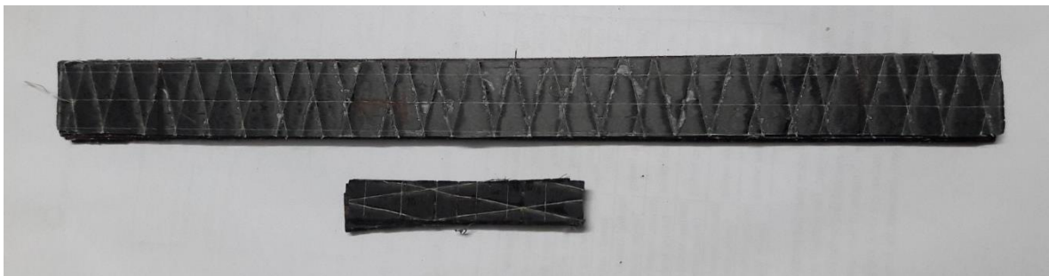
Figure 3.8 : Tensile and flexural rectangular specimens
